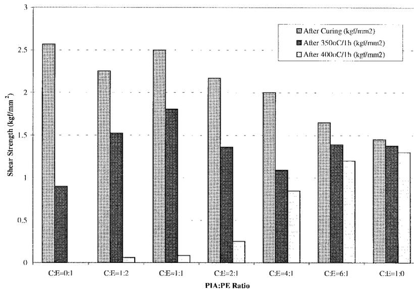
Fig. 5. Shear strength versus PIA to PE ratio for adhesives exposure to various thermal processes.
