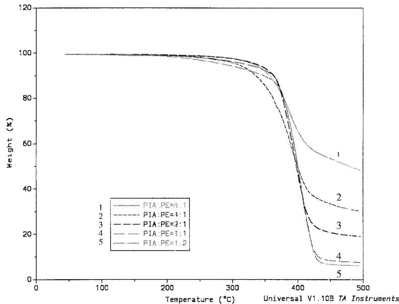
Fig. 1. TGA scan of thermally reworkable adhesives.
