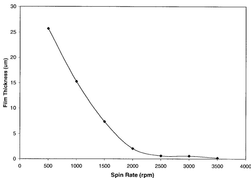
Fig. 3. Plot of adhesive thickness versus spin rate of developed adhesive with PIA:PE ratio of 1:1 (spin time = 30 s).
