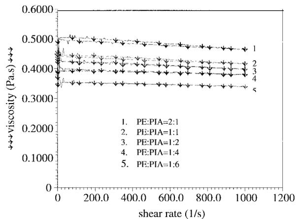
Fig. 2. Plot of viscosity versus shear rate for various PIA to PE ratios.
