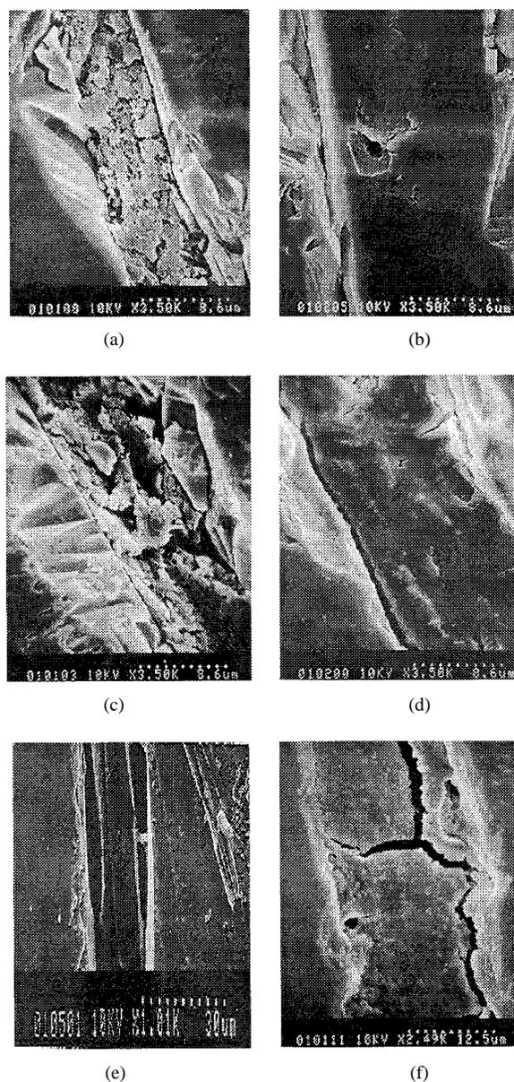
Fig. 6. SEM microstructure cross section analysis. (a), (c), (e) are the developed PIAE adhesives (PIA:PE = 1:1) exposed to curing temperature, 350  $^{\circ}\text{C}/1$  h, and 400  $^{\circ}\text{C}/1$  h, respectively. (b), (d), (f) are the commercial PIA adhesives exposed to curing temperature, 350  $^{\circ}\text{C}/1$  h, and 400  $^{\circ}\text{C}/1$  h, respectively.
