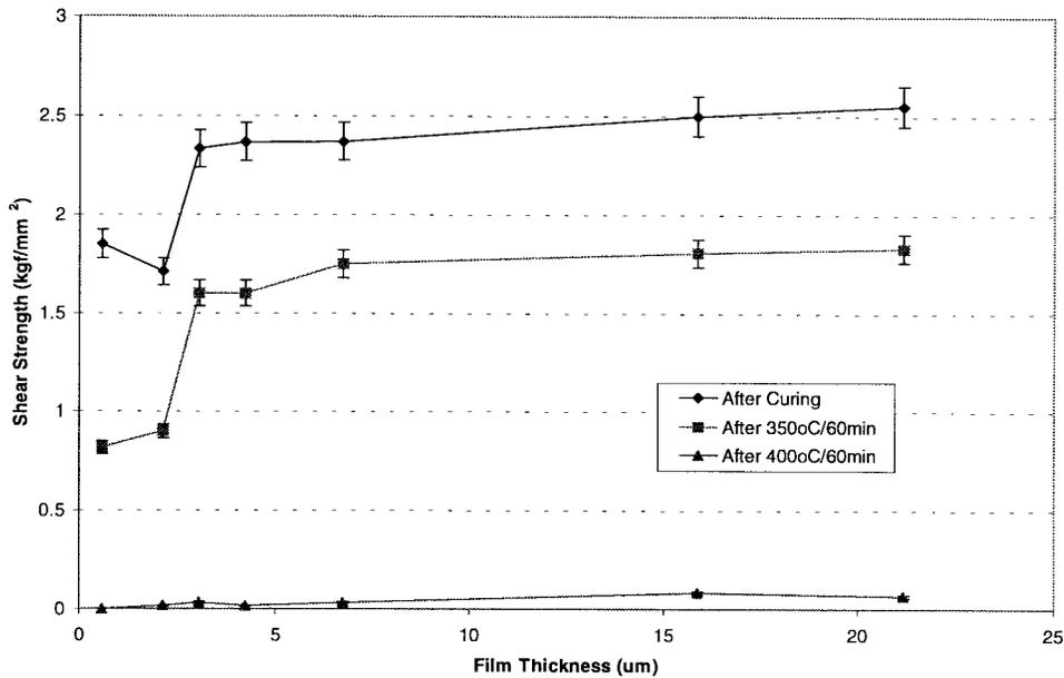
Fig. 4. Shear strength versus film thickness for adhesives (PIA:PE = 1:1) exposure to various thermal process.
