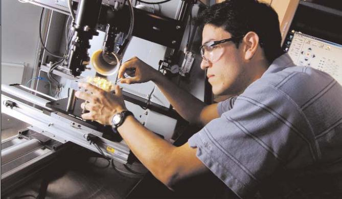
machining fabrication to build electrical and mechanical systems at the micron scale — one-millionth of a meter. Although MEMS was originally developed for the integrated circuit industry, it's an attractive platform for medical devices because mechanical, sensory and computational functions can be placed on a single chip.)
