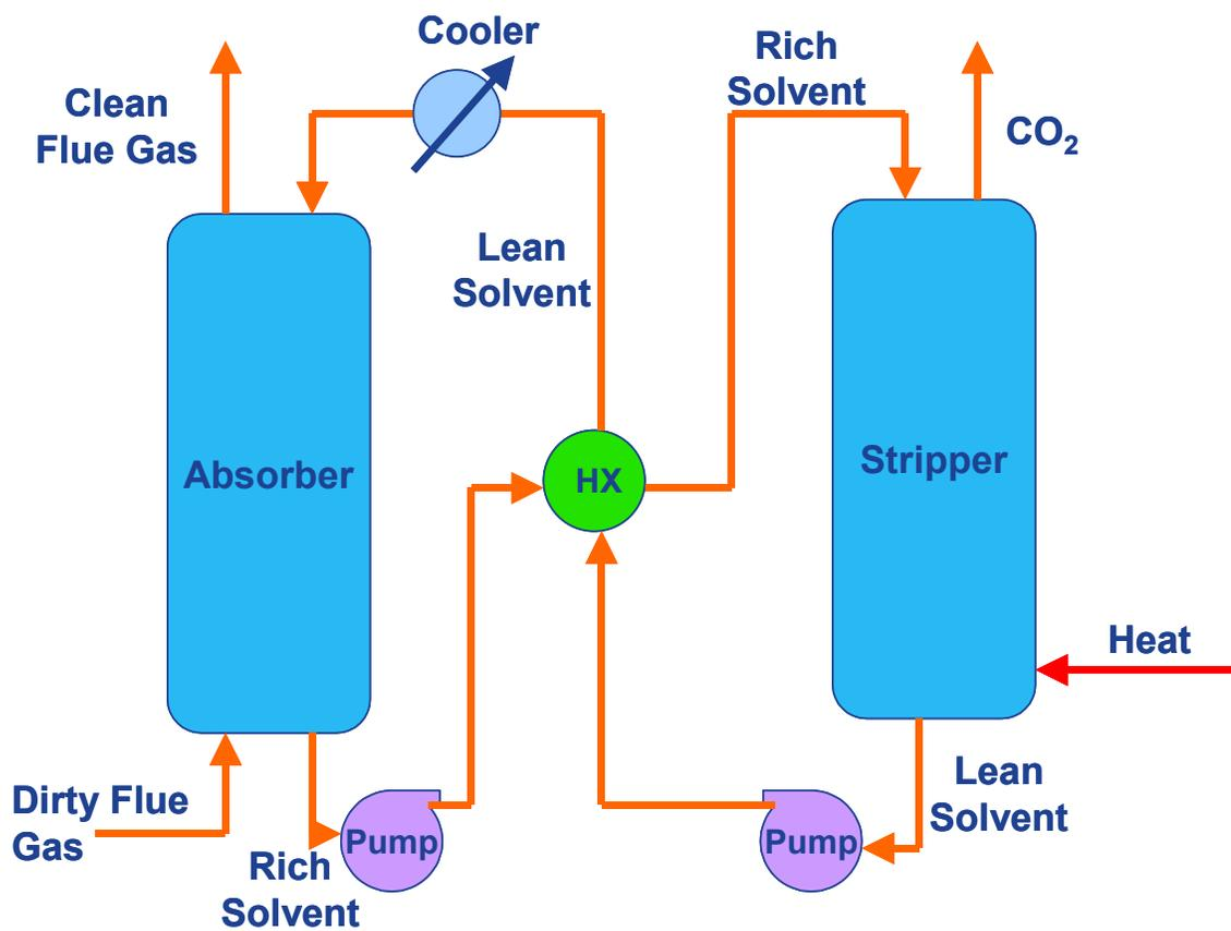
Figure 3: Schematic of post-combustion chemical absorption (Schwerman et al, 2005)
