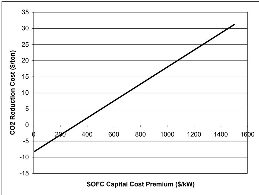
**Figure 15: Sensitivity analysis of CO<sub>2</sub> reduction cost to capital cost premium over pulverized coal powered steam turbine with coal price of \$1.5 per MMBTU and Natural gas price of \$6 per MMBTU**
