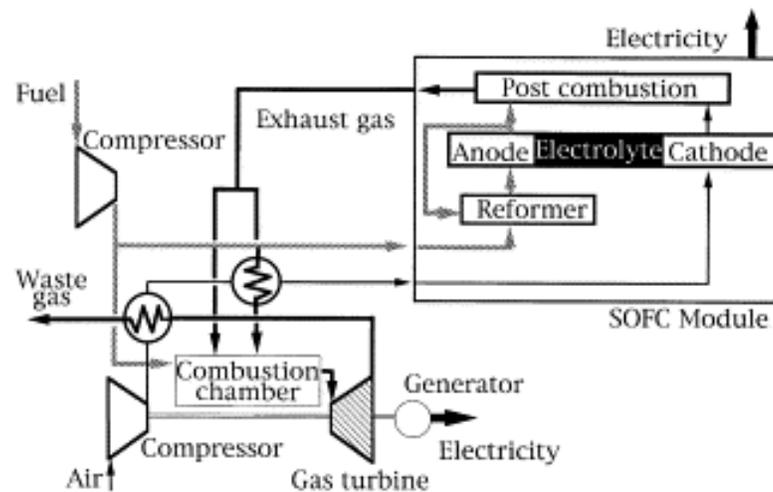
**Figure 14: Solid oxide fuel cell combined cycle system diagram (Tanaka et al, 2000)**
