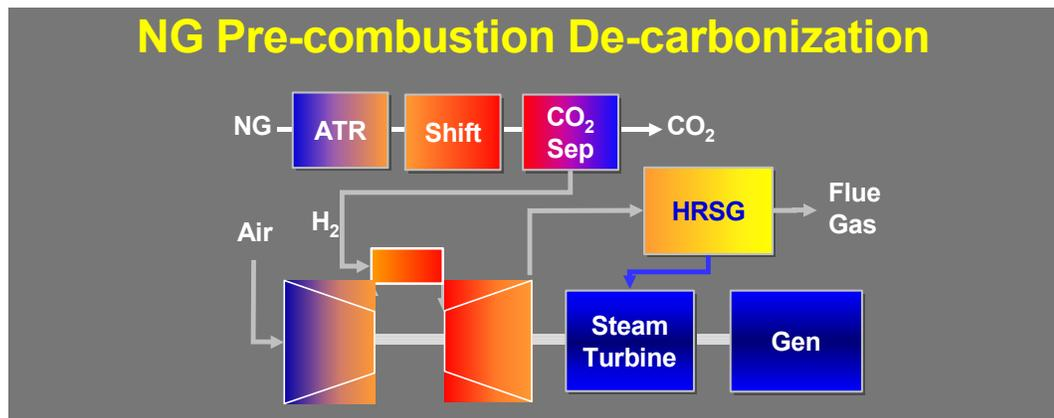
Figure 7: Schematic of ATR-GTCC with CO<sub>2</sub> capture (Schwerman et al, 2005)
