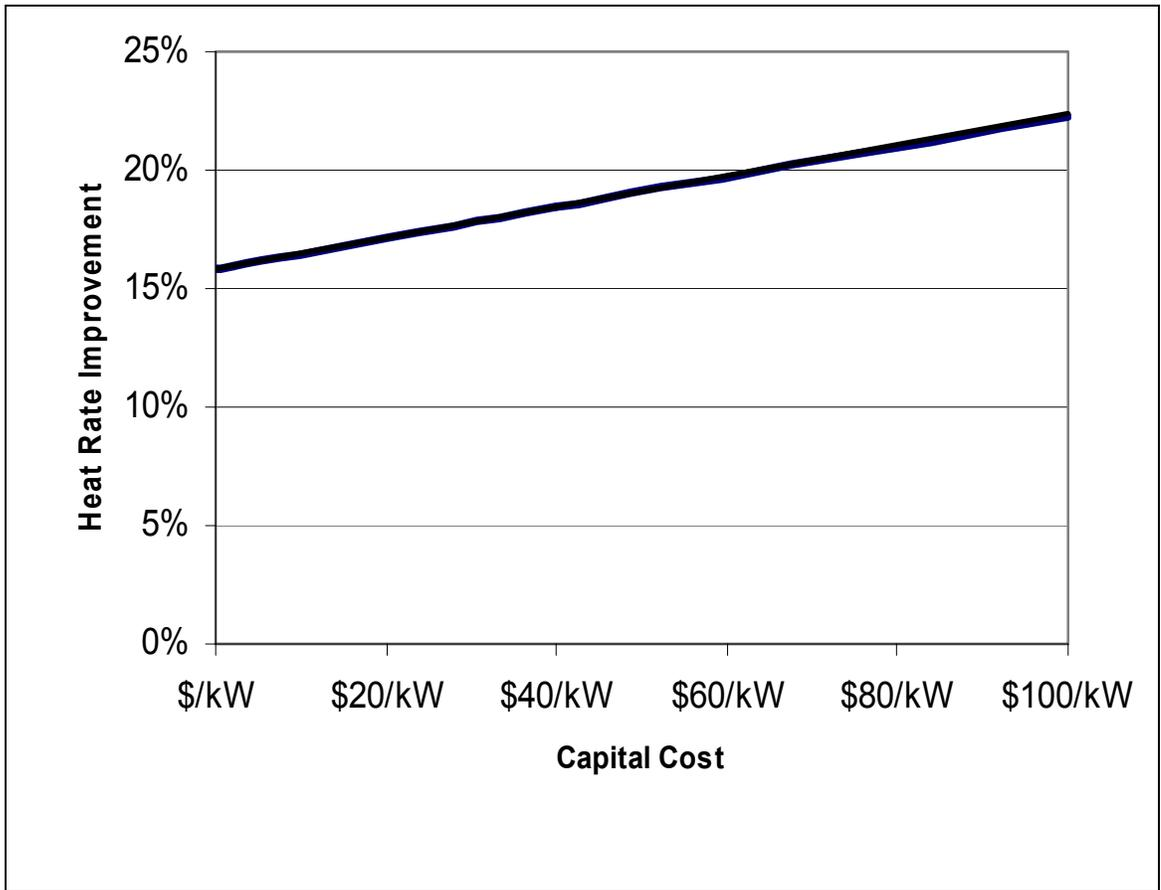
**Figure 12: Variable capital cost analysis for fuel switching with efficiency improvements**
