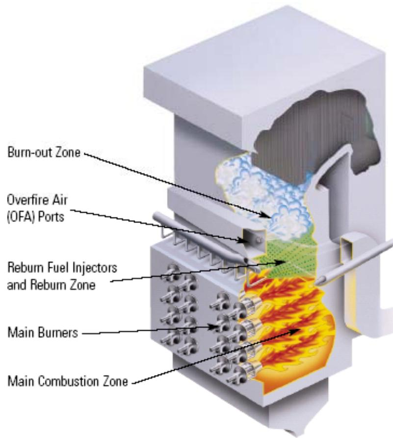
**Figure 9: Wall-fired Boiler with Reburn, (Schwerman et al, 2005)**
