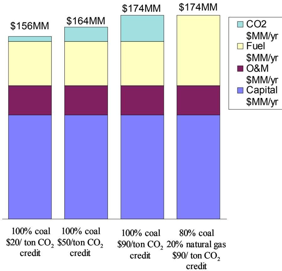
**Figure 11: Comparison of coal boiler with and without natural gas reburn and CO<sub>2</sub> credits; coal price of \$1.5 per MMBTU, and Natural gas price of \$6 per MMBTU.**
