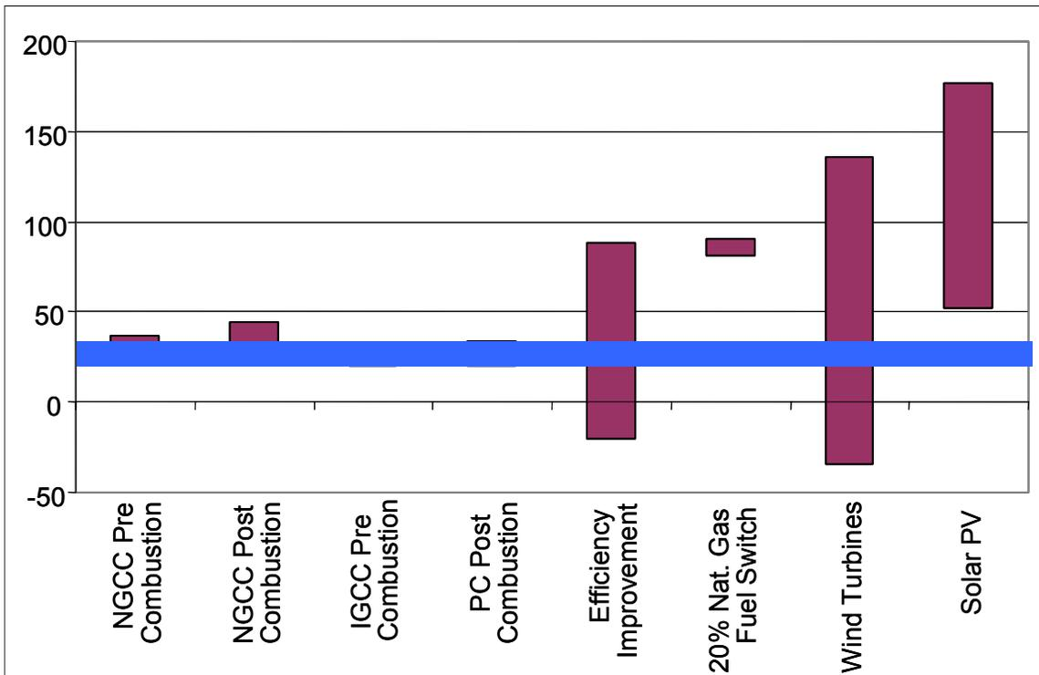
Figure 13: CO<sub>2</sub> Reduction Cost Versus CO<sub>2</sub> Credit Cost
