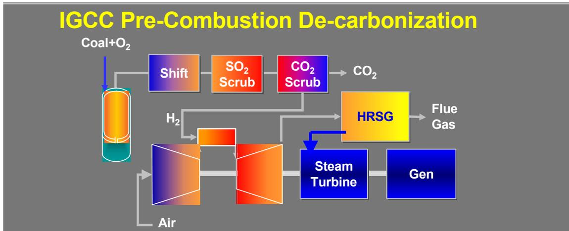
**Figure 5: Schematic of IGCC with CO<sub>2</sub> capture (Schwerman et al, 2005)**
