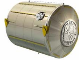
Figure 9: Multi-Purpose Logistics Module (MPLM) is analogous to a Propellant Resupply Module (PRM) for depot resupply.
