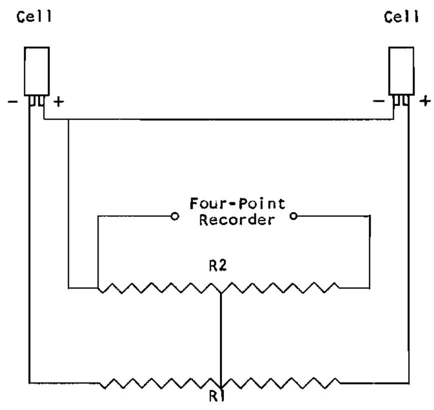
Fig. 4.-Photoelectric Cell Connections
