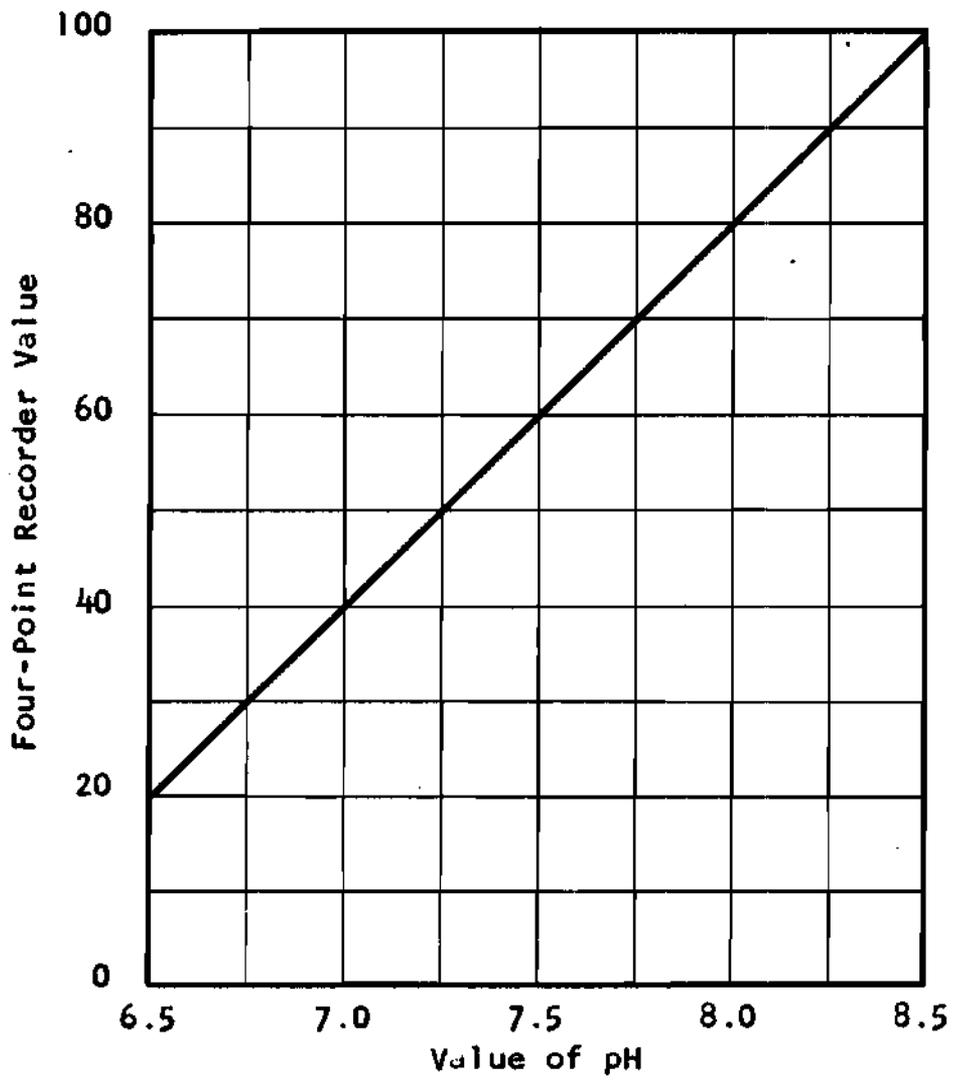
Fig. 1.-Calibration Curve for pH
