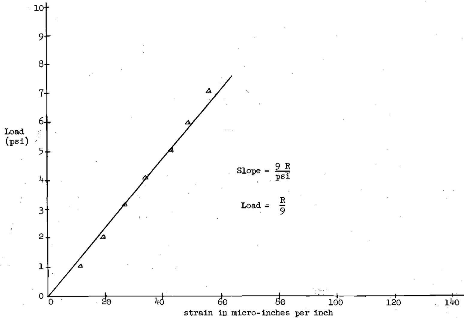
Figure 9. Gauge 2 -- Lateral Load Cell Calibration
