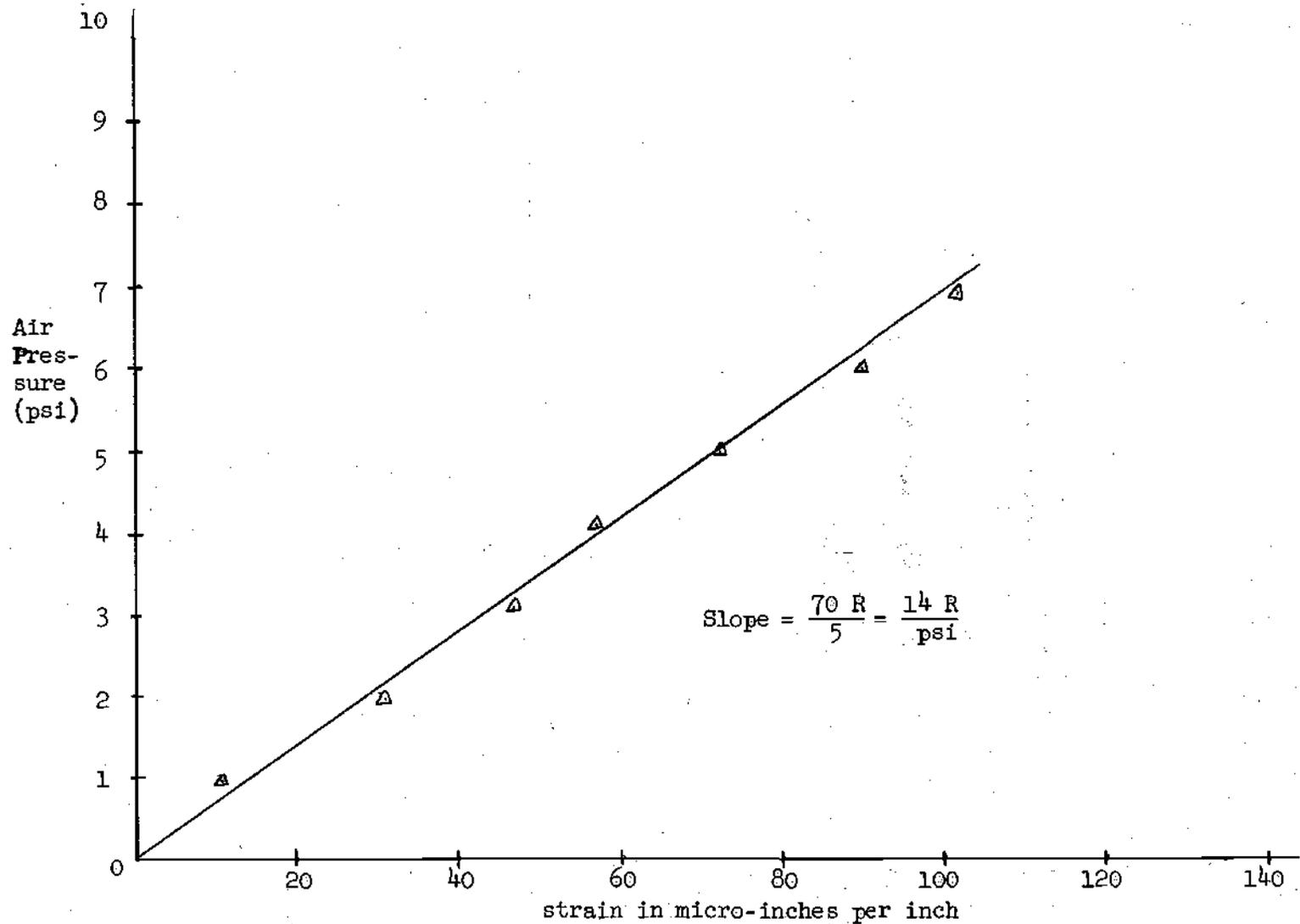
Figure 10. Gauge 3 -- Lateral Load Cell Calibration
