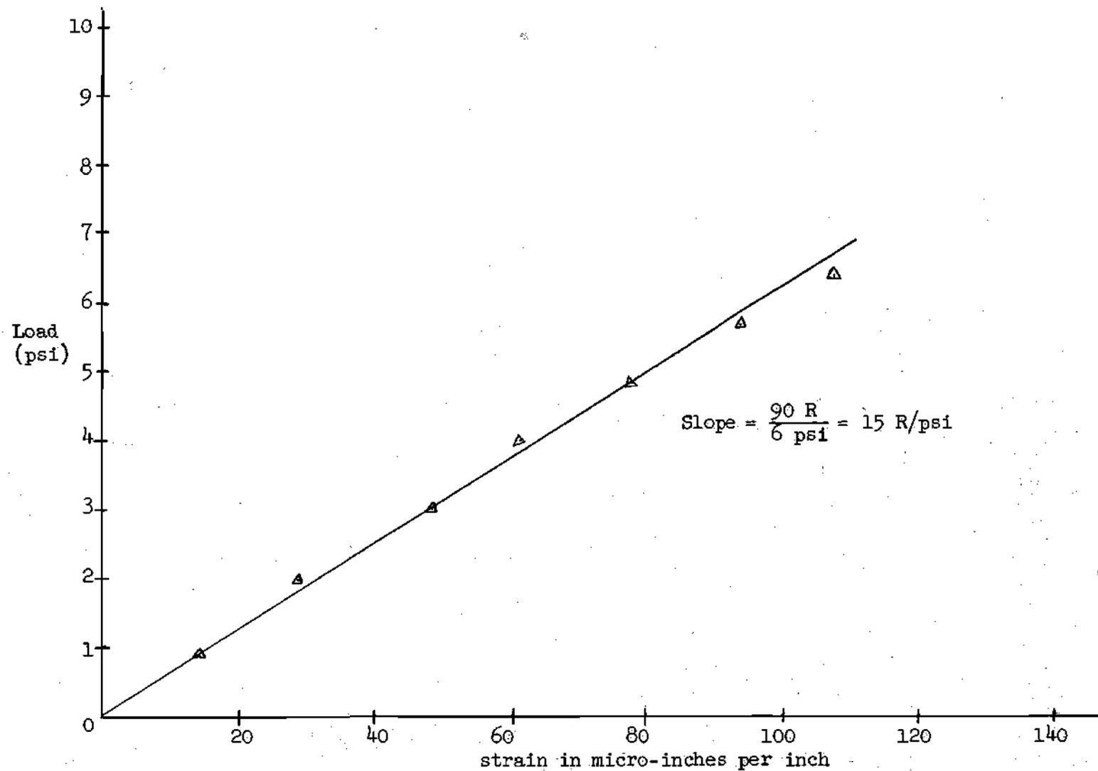
Figure 8. Gauge 1 -- Lateral Load Cell Calibration
