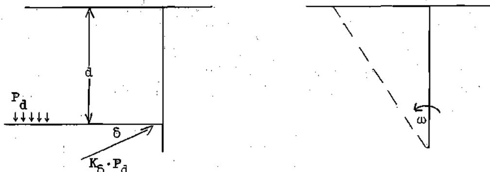
When  $\omega$  is zero,  $K_0$  is equal to  $K_0$  and has the value of  $0.5 \sec \delta$ , this being the lower limit. As  $\omega$  increases, the pressure on the side of the wall increases until a critical value is reached beyond which further increase in  $\omega$  will not increase  $K_0$ . This maximum pressure is the ultimate "passive" pressure.
