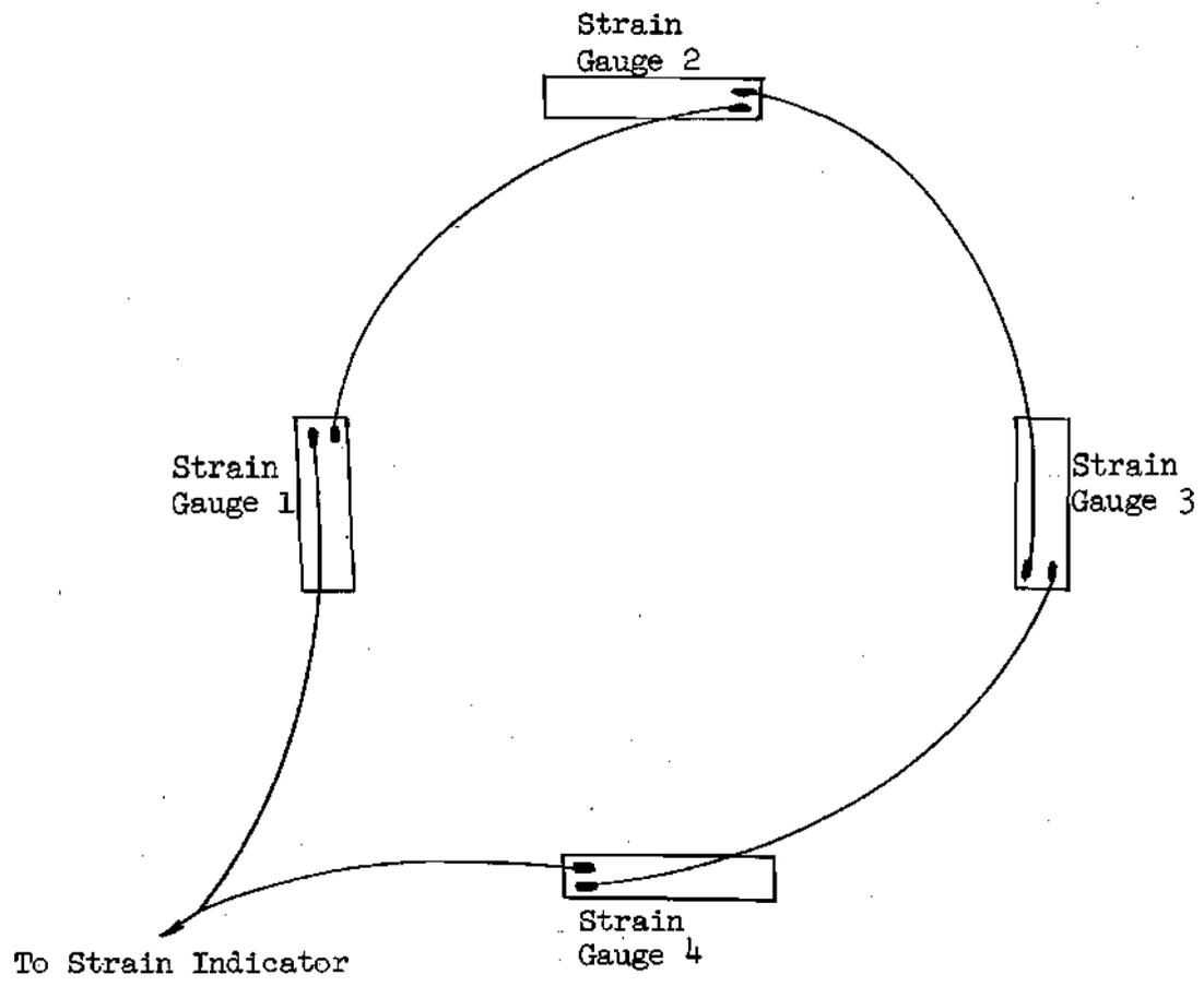
Figure 4. Wiring Diagram for Lateral Load Cells
