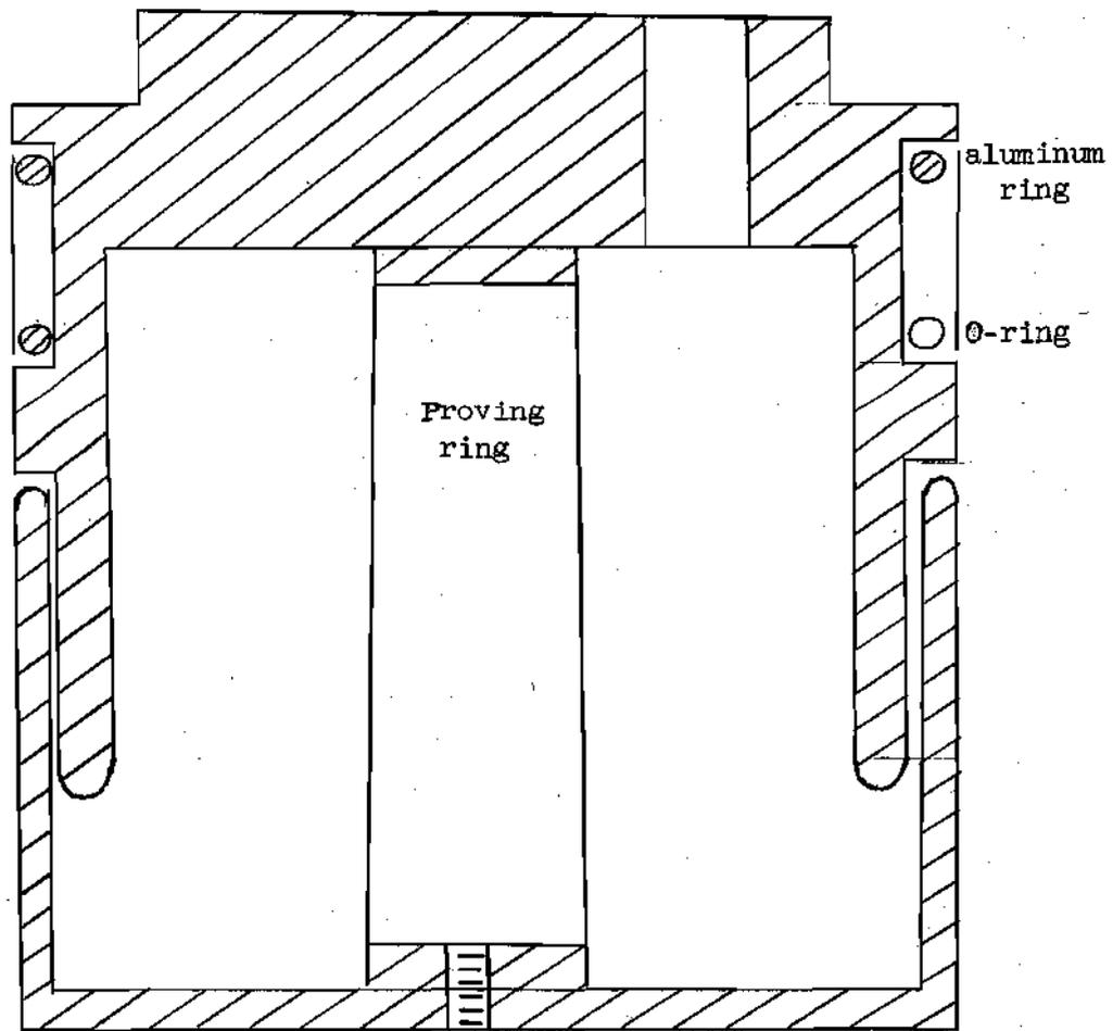
Figure 6. Base Plate Load Cell
