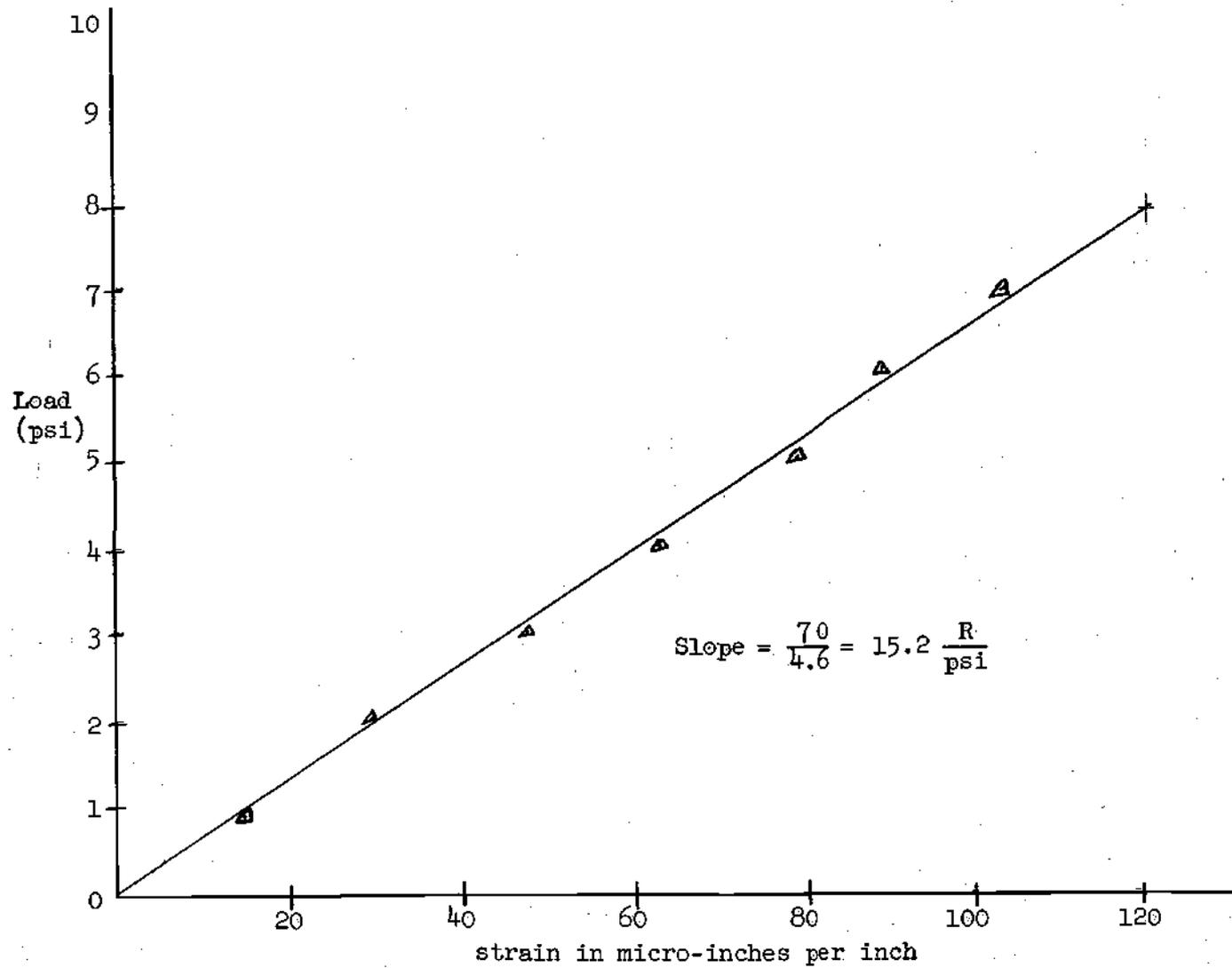
Figure 11. Gauge 4 -- Lateral Load Cell Calibration
