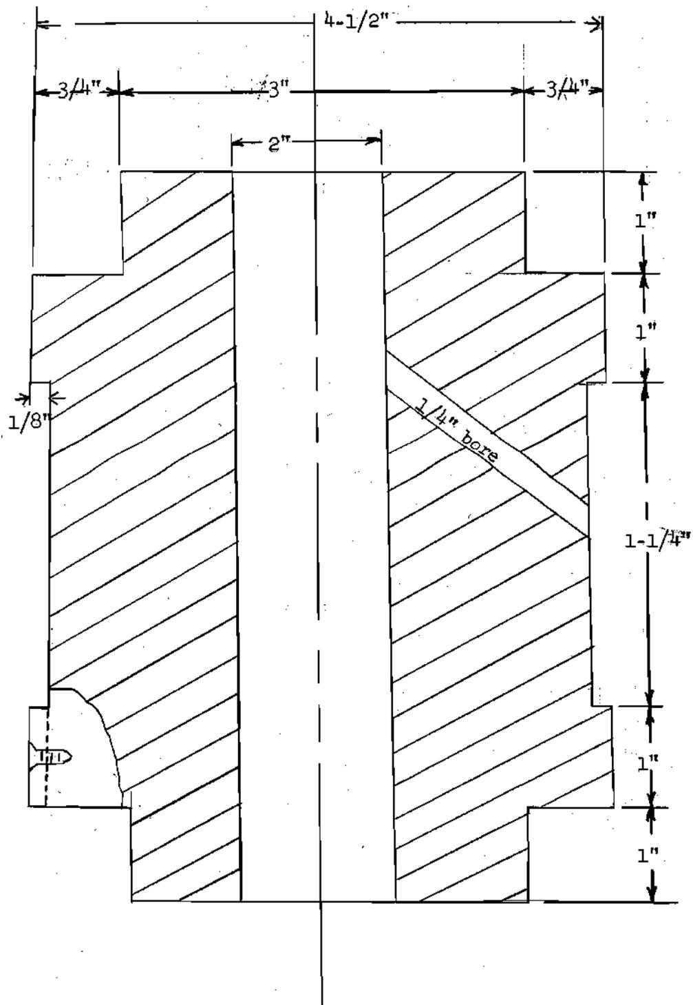
Figure 5. Lateral Pressure Load Cell
