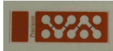
Fig 2. Example three-chamber test slide. The diameter of each chamber measured 7mm. The channel connecting the test and start chambers measured 8mm long with an average width of 2.3mm.
