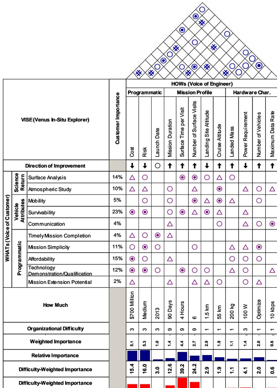
Figure 8. Quality Function Deployment (QFD) for VISE.
