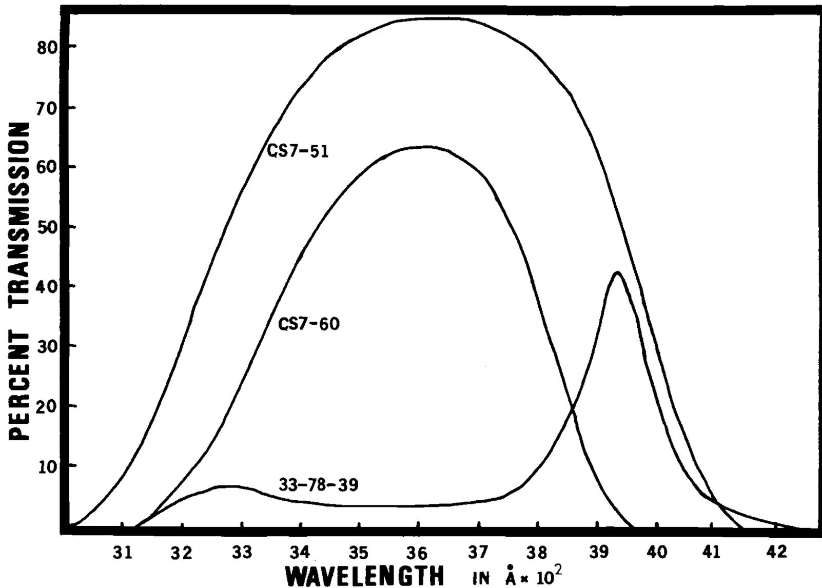
Figure 2. Percent Transmission of Experimental Filters
