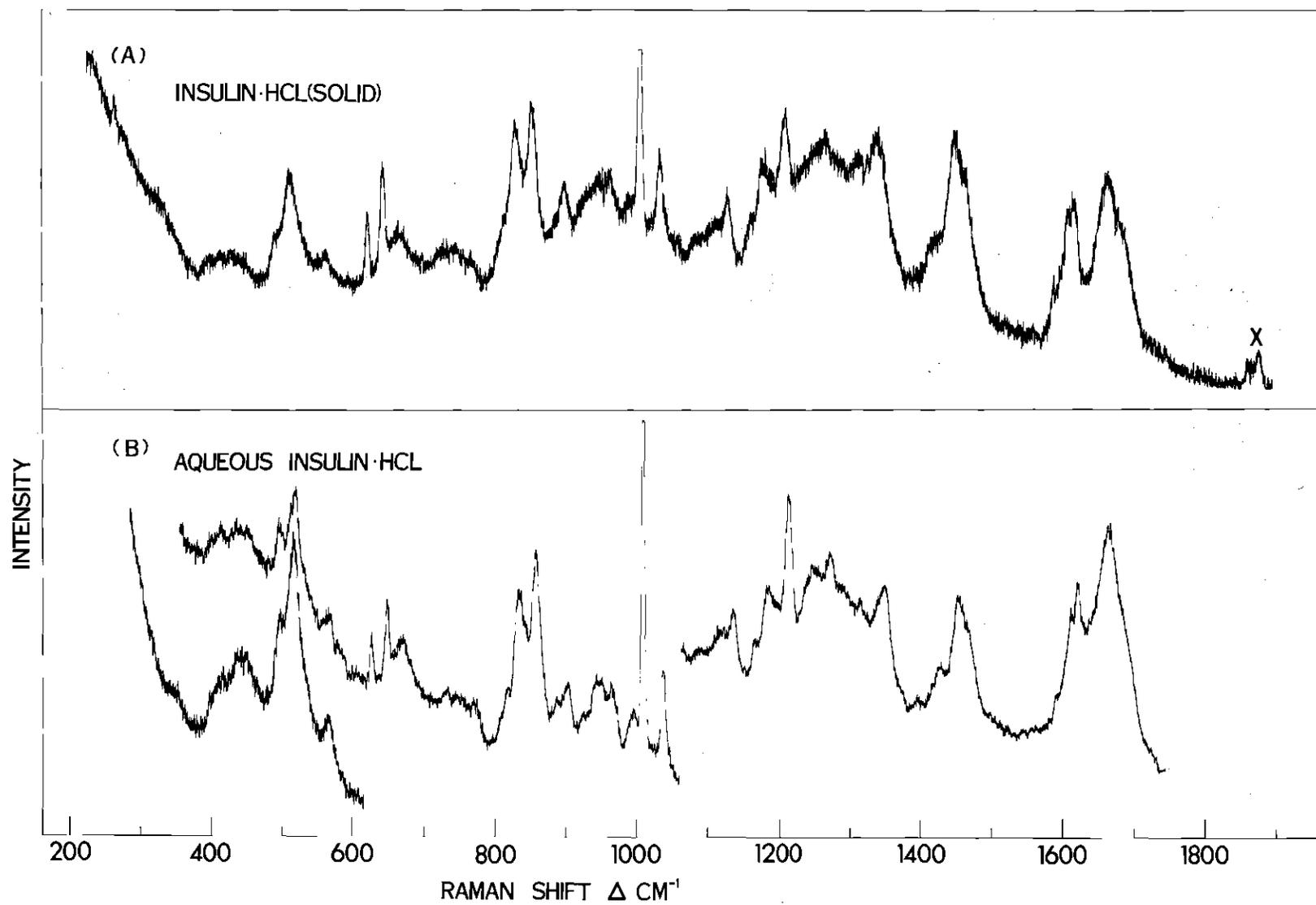
Figure 9. Comparison Between the Raman Spectra of Insulin in the Solid State and in Solution
