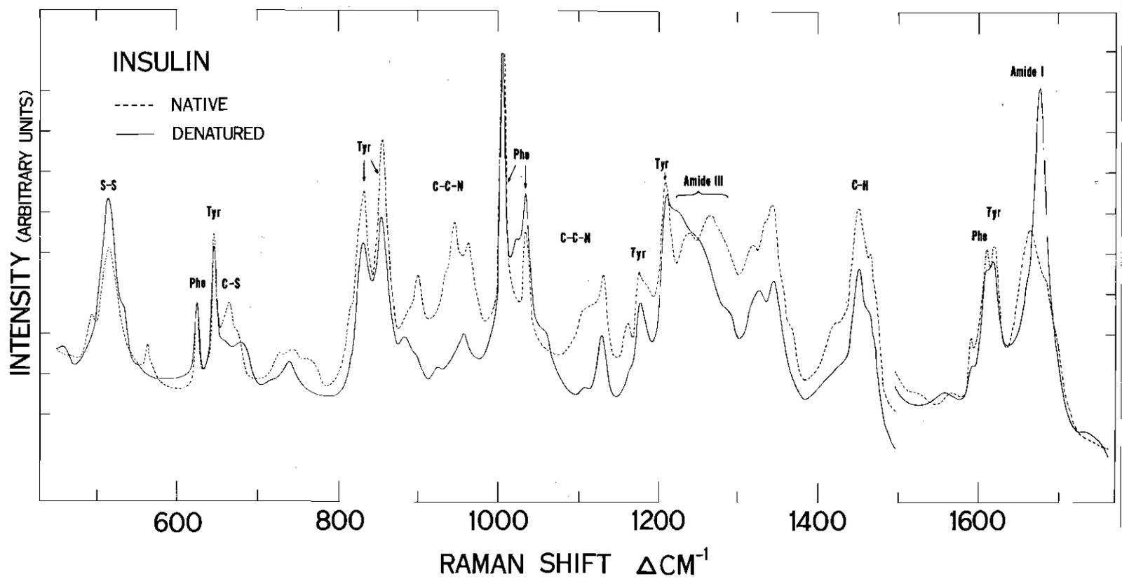
Figure 6. Superimposed Comparison Between the Spectra of Native and Denatured Insulin (redrawn from Fig. 5)
