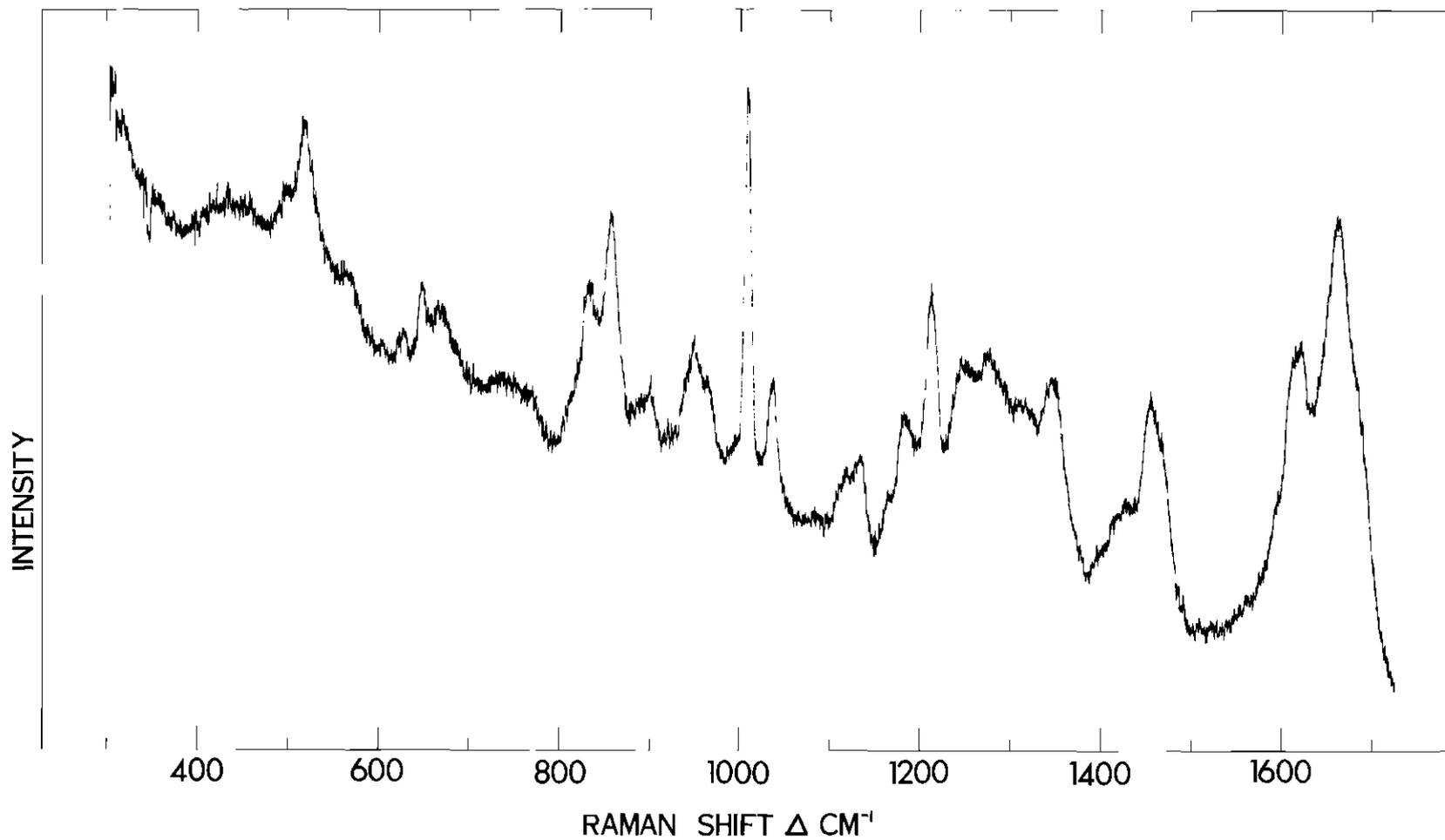
Figure 10. Raman Spectra of Aqueous Insulin at pH 8.50
