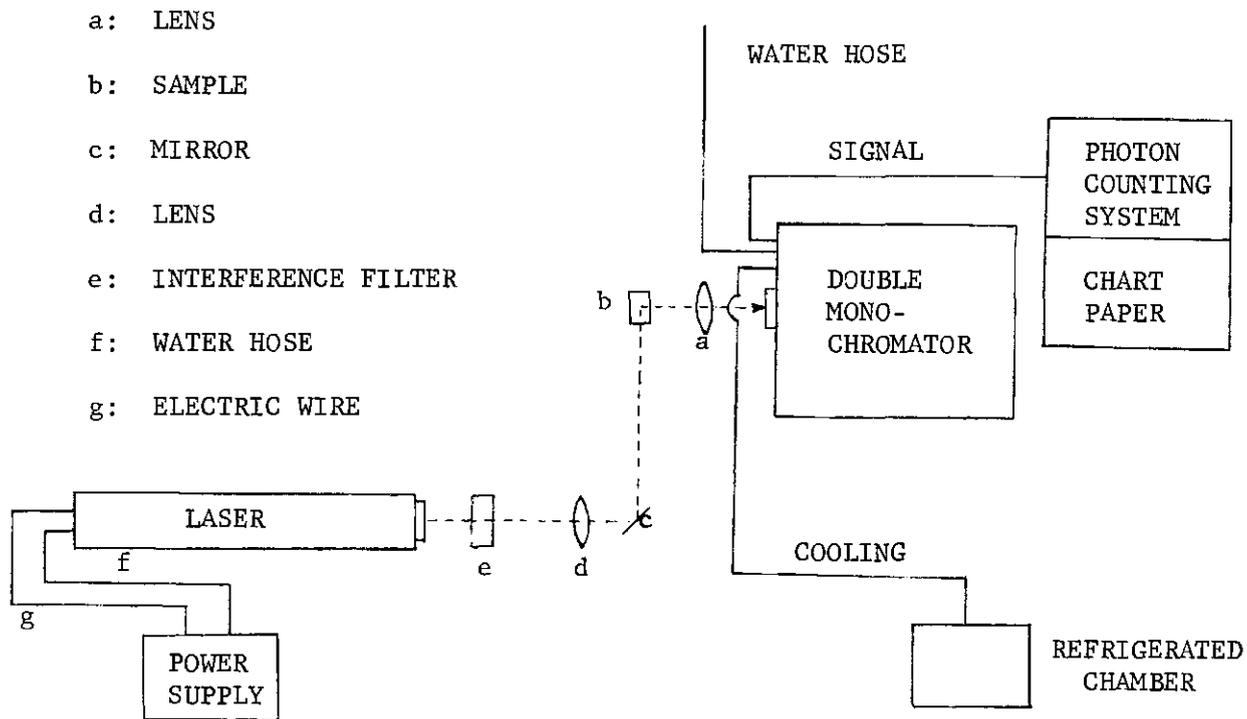
Figure 3. The Arrangement of the Various Parts of the Laser Raman System
