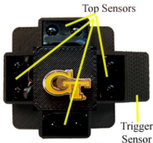
Figure 1. The Gesture Watch prototype with four sensors on the top of the device and a fifth placed horizontally to act the trigger for gesture recognition.
