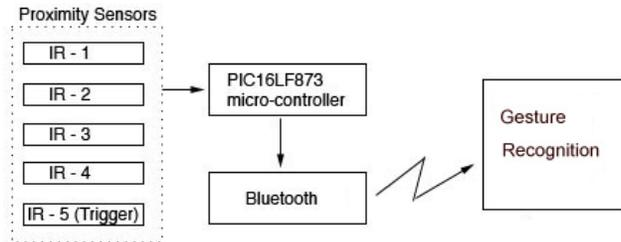
**Figure 12. The Gesture Watch is composed of a PIC microcontroller which reads data from 5 IR proximity sensors. The PIC sends the sensor data wirelessly using a Bluetooth module to a remote computer which interprets the data as gestures.**
