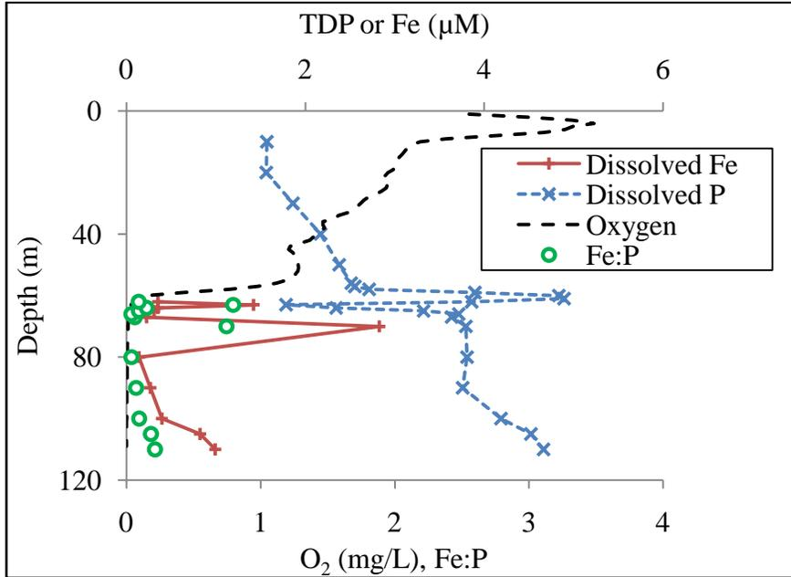
Figure 2. Total Dissolved P (TDP), Fe, Oxygen (O<sub>2</sub>), and Fe:P ratios with depth in April CTD cast. The redox boundary is defined by the O<sub>2</sub> depletion at about 60 m. A sharp increase in P is also observed at this depth, followed by a similar increase in Fe several meters later.
