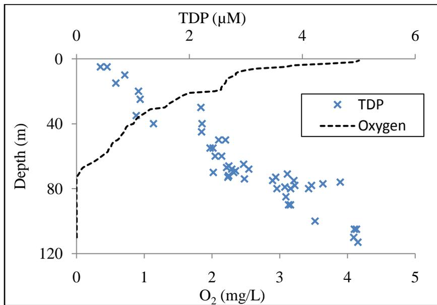
Figure 1. Total dissolved phosphorus (TDP) and Oxygen (O<sub>2</sub>) with depth in a July CTD cast. The redox boundary is defined by the O<sub>2</sub> depletion at about 75 m. A sharp increase in P is also observed at this depth.
