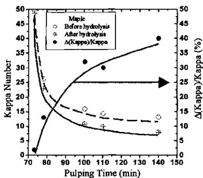
Fig. 4 Kappa number reduction through hydrolysis for the maple pulps obtained at different cooking times.
