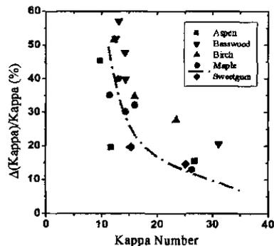
Fig. 5 The correlation between the relative kappa number reduction through hydrolysis and the pulp kappa number for five North American hardwood pulps.
