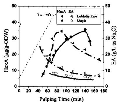
Fig. 1 Time-dependent HexA in pulps and EA in the pulping liquor during conventional kraft pulping .
