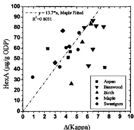
Fig. 6 The correlation between HexA content of pulps and the kappa number reduction through hydrolysis.
