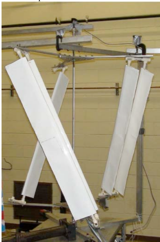
Figure 1: Vertical Axis micro Wind Turbine testbed at the Georgia Tech 42” Wind tunnel.
