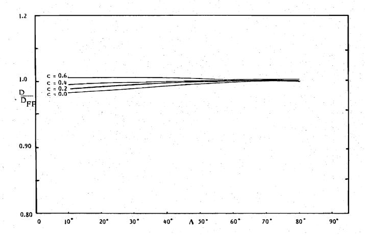
Figure 9. Skin friction drag, normalized with the equivalent flat plate drag, versus sweep angle for various phase speeds, for a series of waves.
