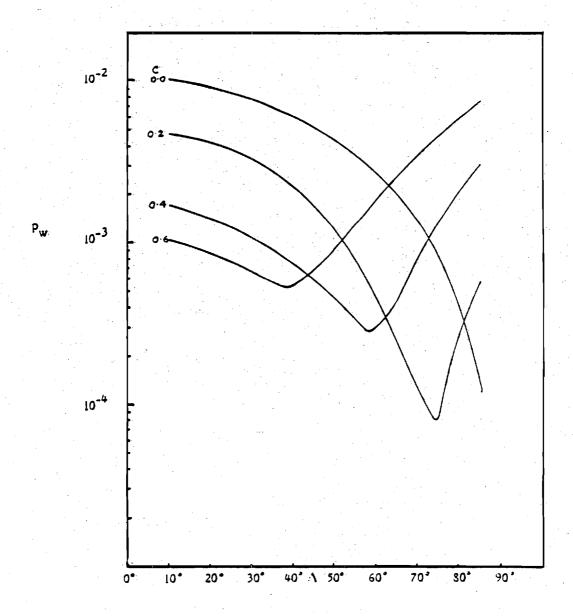
Figure 7. Typical variation of the pressure amplitude at the wall versus sweep angle for turbulent flow.
