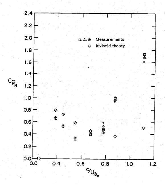
Figure 2. The variation of the pressure coefficient with the phase speed, close to the surface of a water-wave (from Reference 8).
