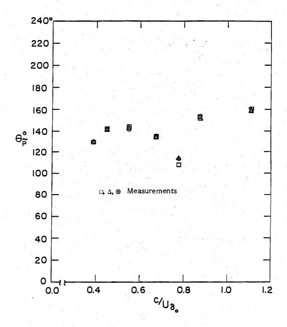
Figure 3. The location of the maximum pressure, in degrees upstream of the crest, for the case of the water-wave (from Reference 8).
