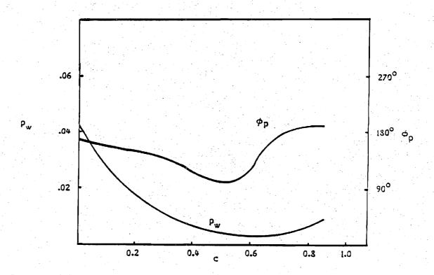
Figure 1. The amplitude of the pressure oscillation and the location of the maximum pressure (degrees upstream of the crest) versus the phase speed.
