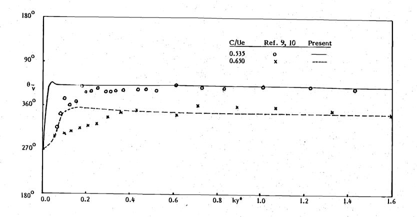
Figure 5. Comparison for calculation and measurement of the phase of normal velocity across the boundary layer.
