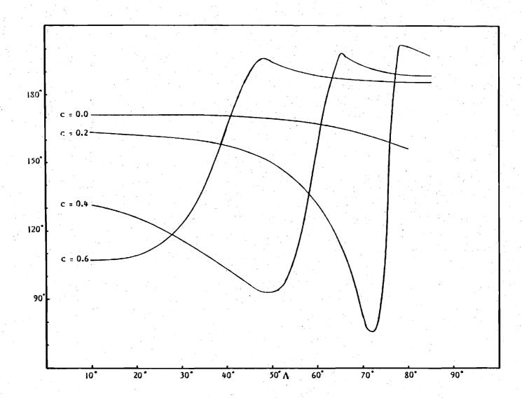
Figure 8. Typical variation of the phase of pressure versus sweep angle for various phase speeds for turbulent flow over a wavy wall.
