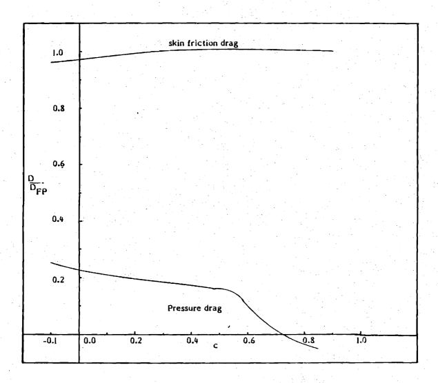
Figure 6. Pressure drag and skin friction drag for various phase speeds for a series of two-dimensional waves.
