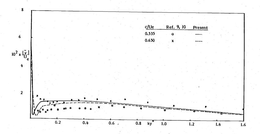
Figure 4. Comparison of calculation and measurement for normal velocity perturbation across the boundary layer.
