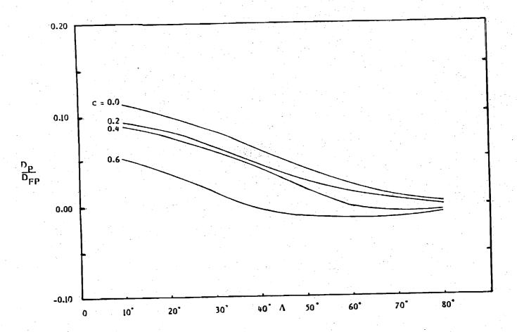
Figure 10. Pressure drag, normalized with the equivalent flat plate drag, versus sweep angle for various phase speeds, for a series of waves.
