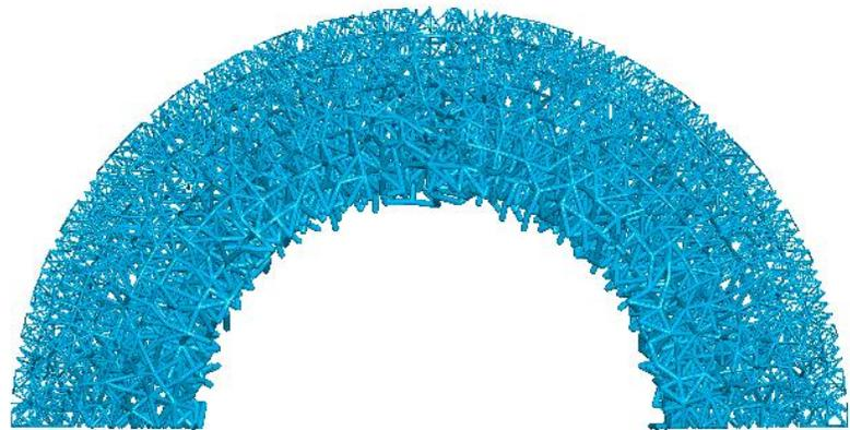
Figure 2. An example of cylindrical graded cellular structures (top view)
