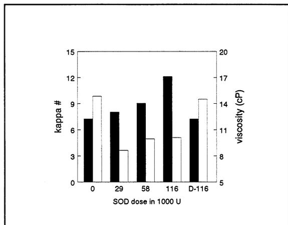
**Figure 5. Superoxide dismutase treatments of active biobleaching conditions of laccase HBT. D-116 is thermally denatured SOD. Solid bar is kappa number, and open bar is viscosity.**
