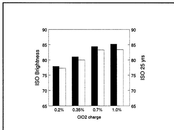
**Figure 4. Chlorine dioxide brightening of L(EOP)LE pulp with different ClO<sub>2</sub> charges. Solid bar is ISO brightness, and open bar is ISO brightness after thermal reversion equal to 25 years.**
