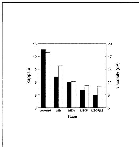
**Figure 2. The effect of reinforced alkaline extraction and two stages of laccase HBT treated softwood kraft Post- $O_2$  industrial pulp. Solid bar is kappa number, and open bar is viscosity.**
