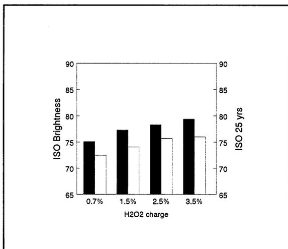
**Figure 3. Hydrogen peroxide brightening of L(EOP)LE pulp with different H<sub>2</sub>O<sub>2</sub> charges. Solid bar is ISO brightness, and open bar is ISO brightness after thermal reversion equal to 25 years.**
