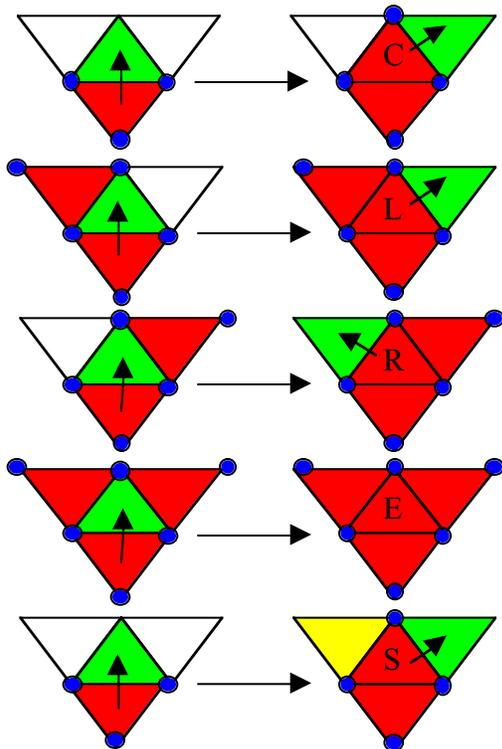
where green identifies the current triangle, yellow identifies a triangle to be put on the stack of future current triangles popped after each E, red identifies previously processed triangles, white identifies triangles not yet processed, and blue identifies previously processed vertices. The resulting sequence of C, L, R, E, or S labels suffices to capture the
