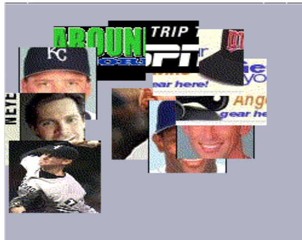
Figure 3.3.2: CWIC is a standalone application using the spiral layout. The collected images are displayed to the user in a circular pattern starting from center to the perimeter to center counterclockwise and back from center to the perimeter to center clockwise. Each image is partially overwritten by another image.
