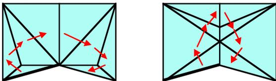
Figure 2: The two meshes have boundaries as triangle-spanning trees, as shown by red arrows and described by the sequence of moves left, right, right, right, left, right.
