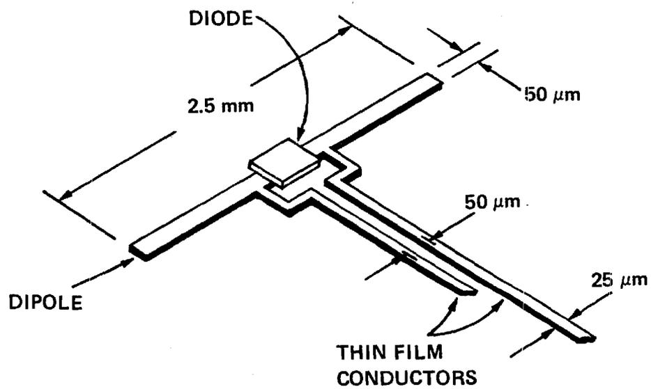
Figure 14. Detail of BRH Probe.
