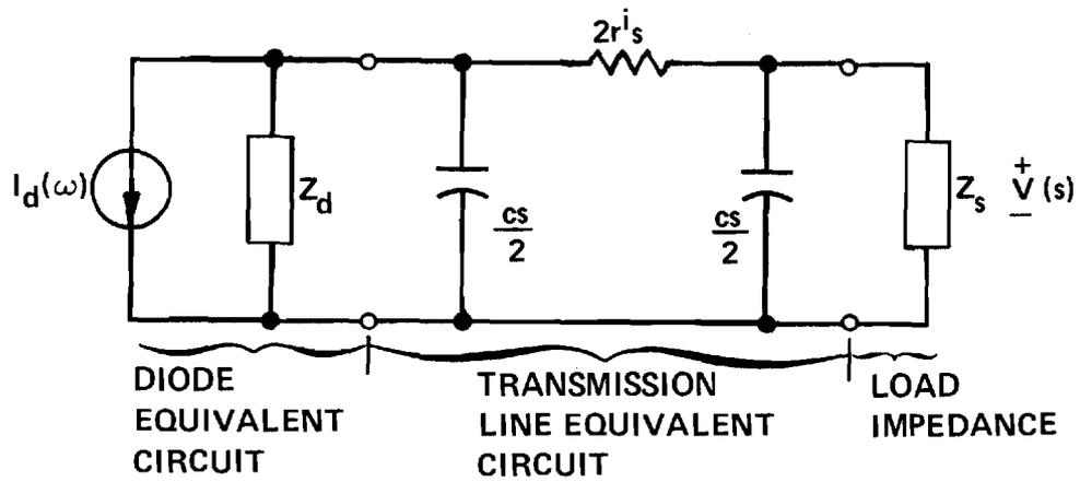
Figure 11. Low-Frequency Output Circuit for Diode, Transmission Line and Termination,  $Z_s$ .
