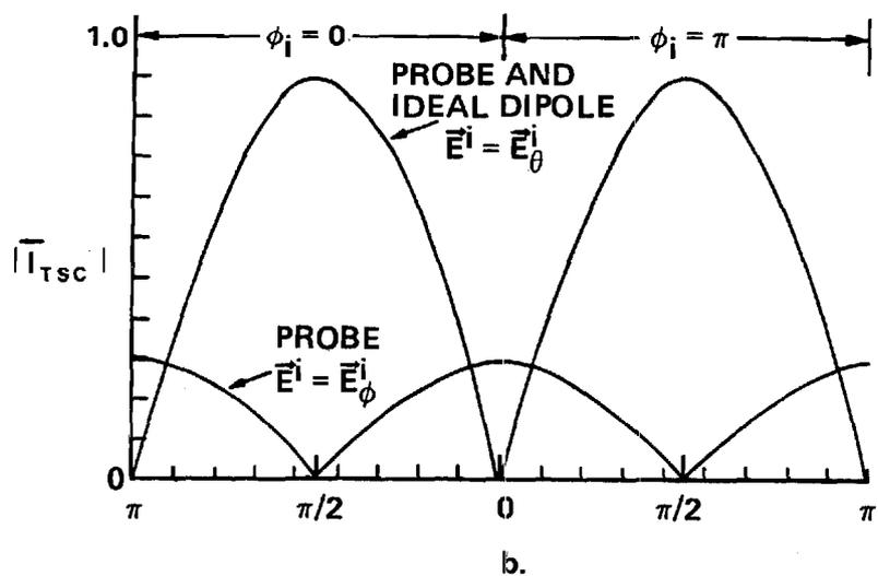
Figure 7. Rectangular Field Patterns in Principal Planes for Probe With Parameter  $\chi = 0.3$ , a.  $\phi_i = \pi/2, 3\pi/2$ , b.  $\phi_i = 0, \pi$ .
