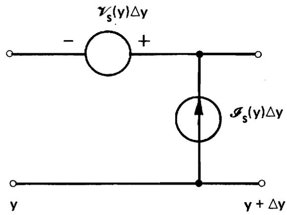
Figure 5. Equivalent Voltage and Current Sources for a Length  $\Delta y$  of the Transmission Line.
