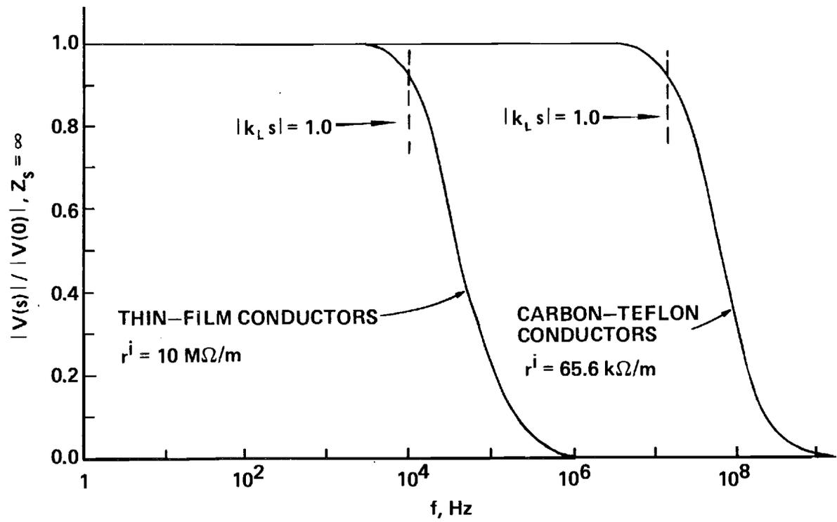
Figure 10. The Voltage Ratio  $|V(s)|/|V(0)|$  as a Function of Frequency for Resistive Transmission Lines Terminated in an Open Circuit,  $Z_s = \infty$ .
