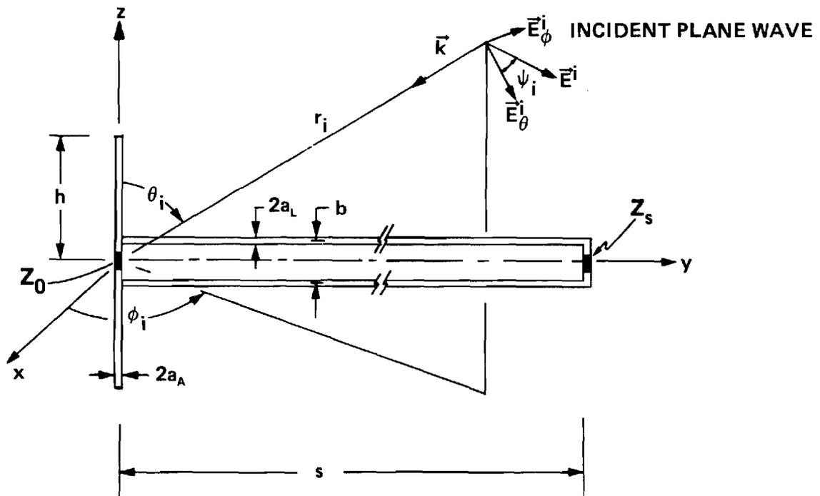
Figure 2. Dipole With Transmission Line in Incident Plane-Wave Field.
