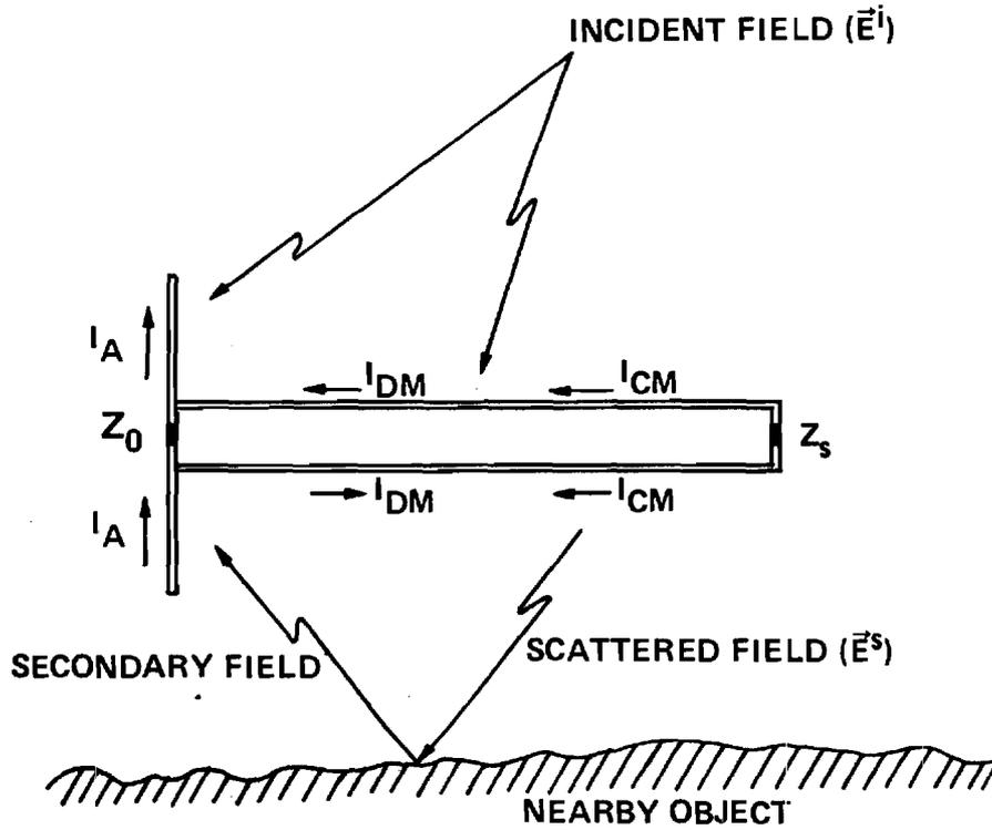
Figure 3. Schematic Diagram Showing Reception of Incident Signal.
