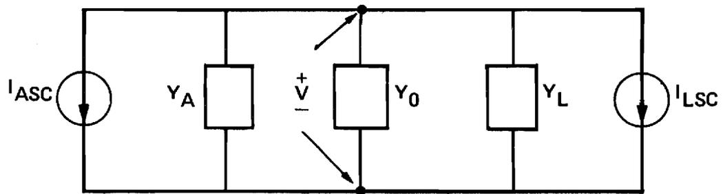
Figure 4. Norton Equivalent Circuit for Dipole-Transmission Line Reception.
