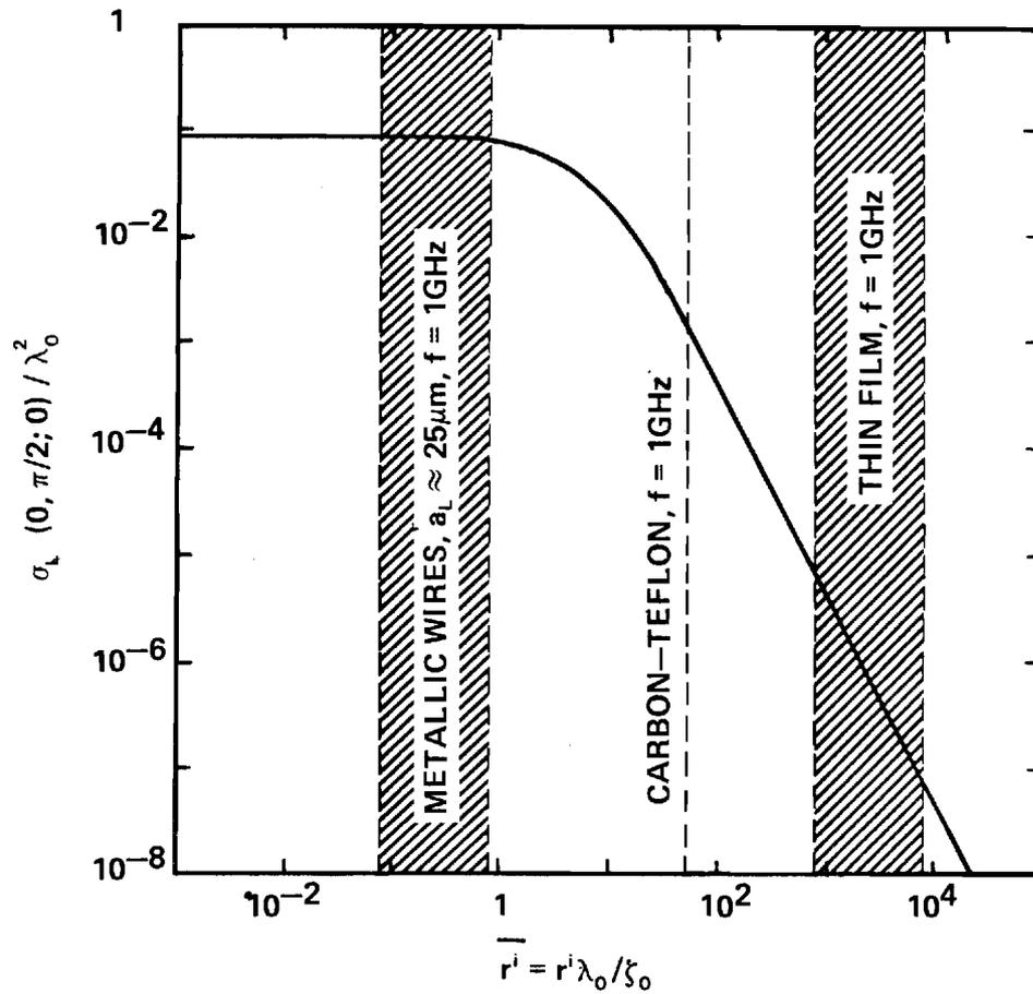
Figure 8. Normalized Total Scattering Cross Section of a One Wavelength Long Transmission Line ( $s/\lambda_0 = 1.0$ ,  $a_0/\lambda_0 = 3.33 \times 10^{-3}$ ) for an Incident Wave With  $\theta_i = 0$ ,  $\phi_i = \pi/2$  and  $\psi_i = 0$ .
