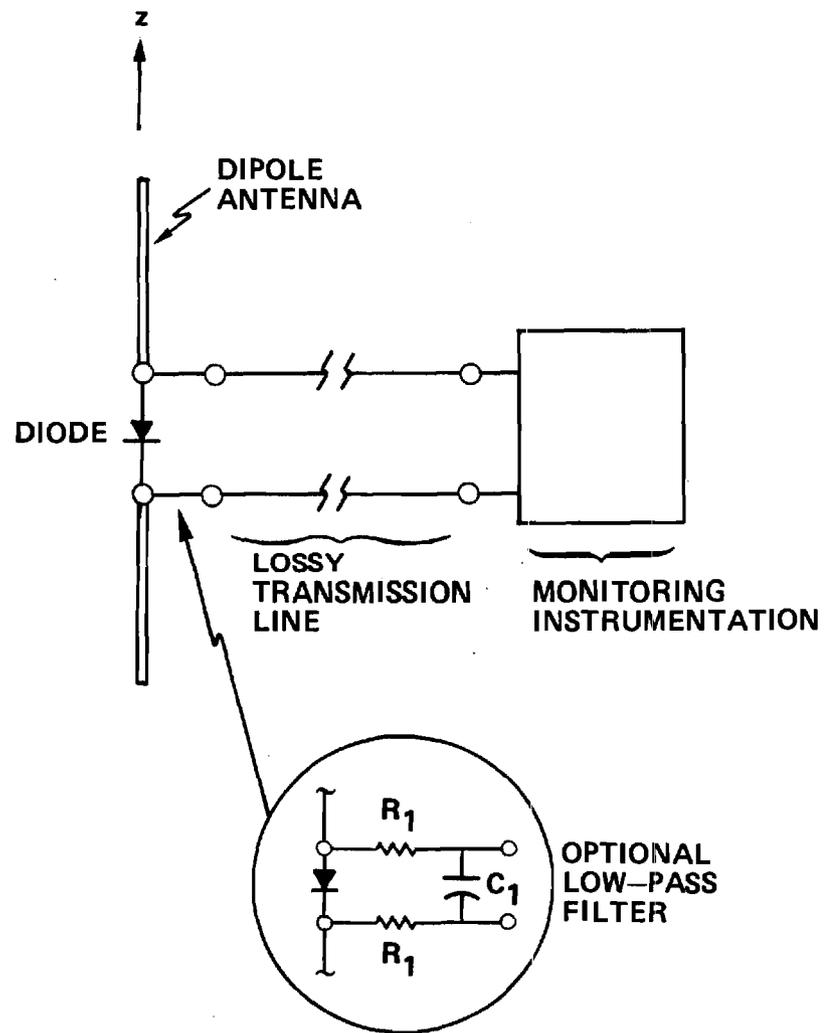
Figure 1. Dipole Receiving Probe.
