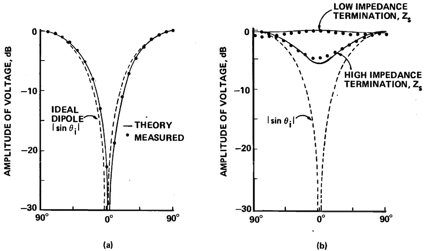
Figure 13. Comparison of Measured and Theoretical Field Patterns in Plane  $\phi_i = \pi/2, 3\pi/2$  With Incident Field  $\vec{E}_\theta$
