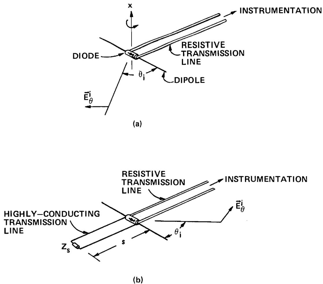
**Figure 12. Detail of Experimental Probe**
