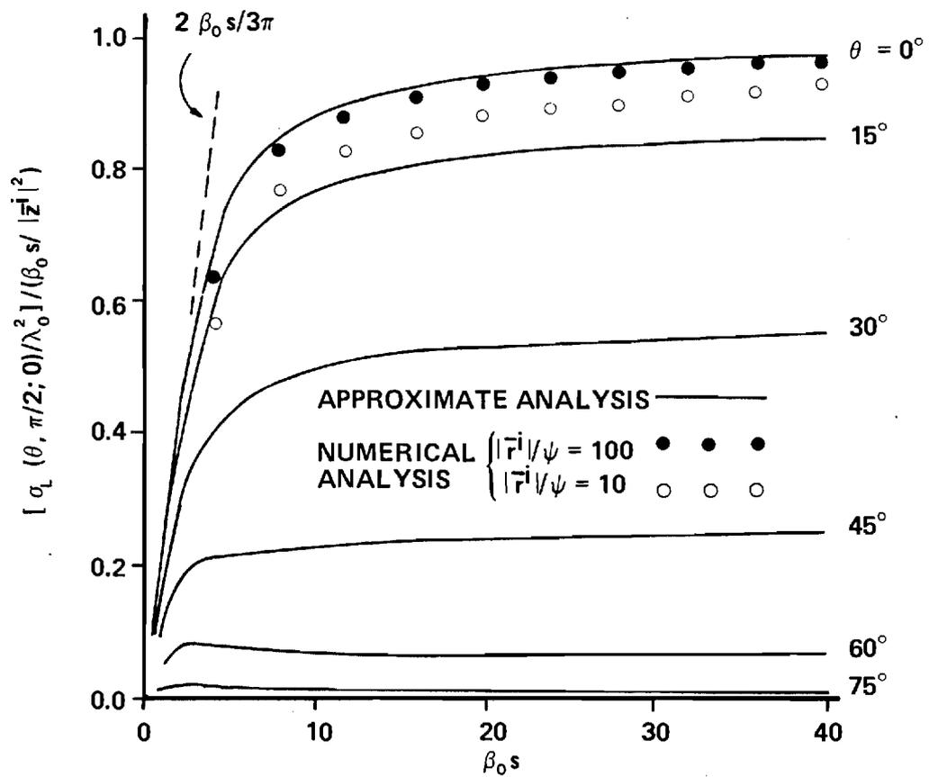
Figure 9. Normalized Total Scattering Cross Section for Transmission Line as a Function of the Electrical Length  $\beta_0 s$ ,  $\phi_i = \pi/2$ ,  $\psi_i = 0$ .
