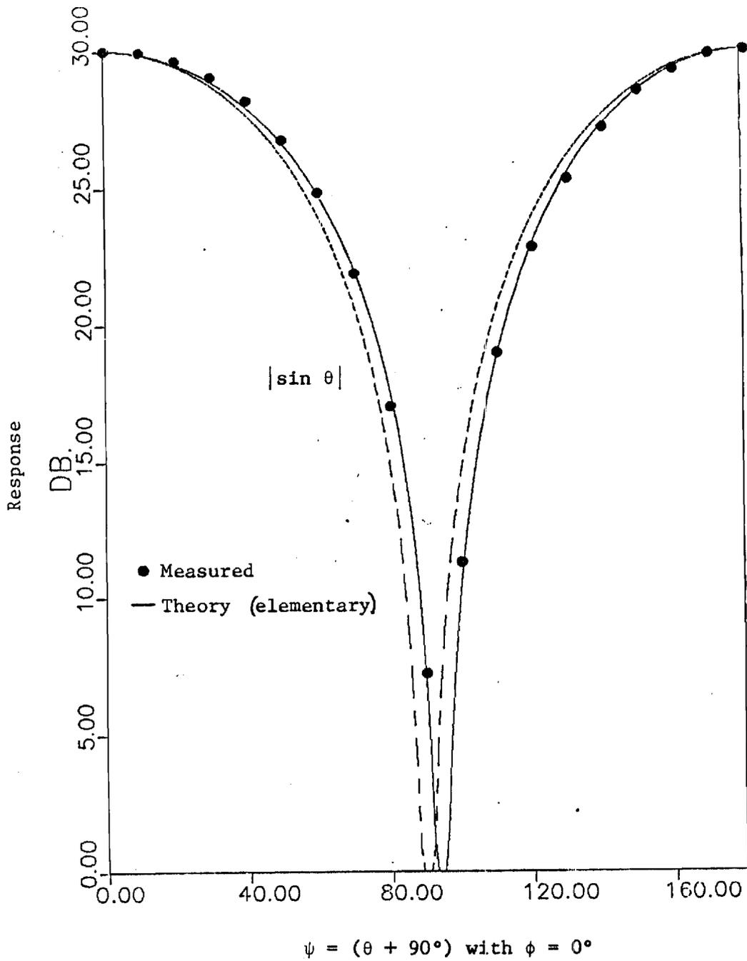
Fig. 2. Field pattern for probe with highly resistive transmission line.
