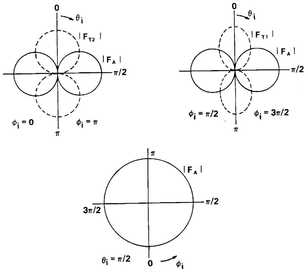
Figure 6. Polar Field Patterns in Principal Planes for Functions  $F_A(\theta_i, \phi_i)$ ,  $F_{T1}(\theta_i, \phi_i)$  and  $F_{T2}(\theta_i, \phi_i)$ .
