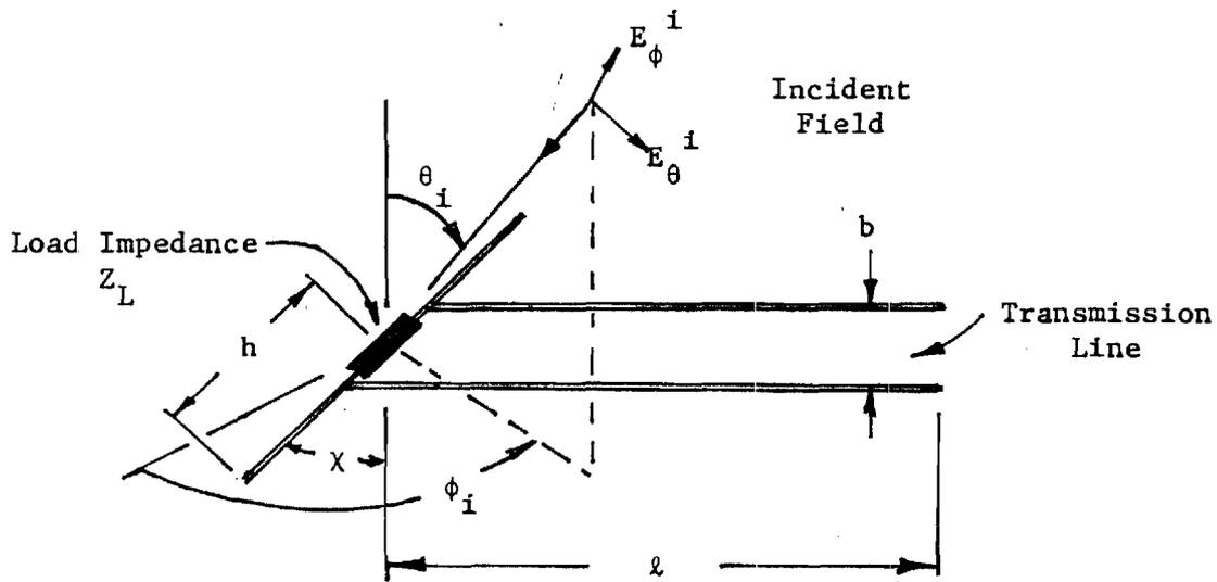
Fig. 1. Geometry of Probe
