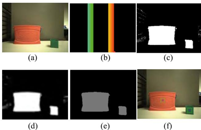
Figure 5. (a) Original Toy Scene Image (b) Back-projected Hue Histogram (c) Histogram Back-projected Image (d) Smoothed Image with Gaussian Filter (e) Binary Thresholded Image (f) Final Toy Objects Detected (center marked with green box)
