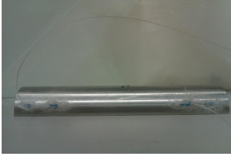
Figure 28. Hemi-cylinder Mounting
