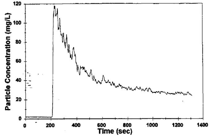
Figure 3. Typical concentration profile for erosion event.
