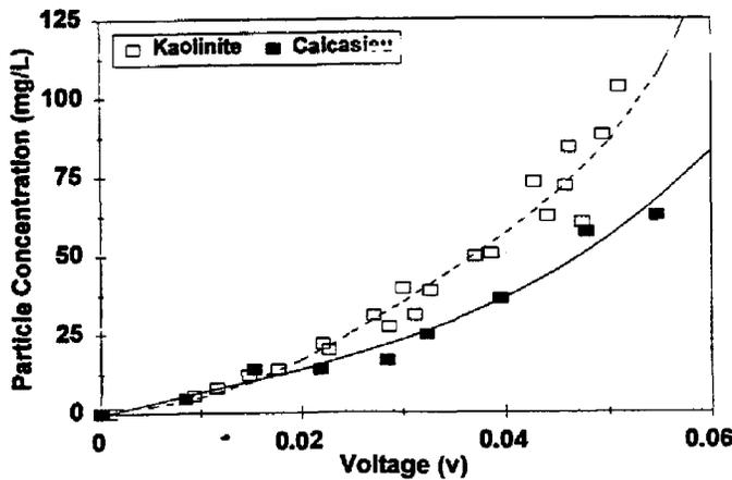
Figure 2. Particle monitor calibration curves.
