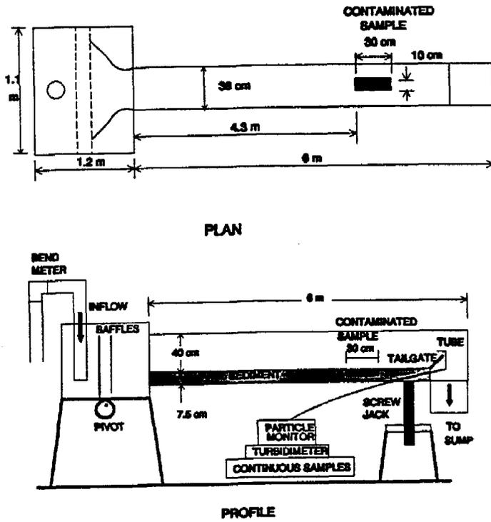
Figure 1. Plan and profile of recirculating flume.
