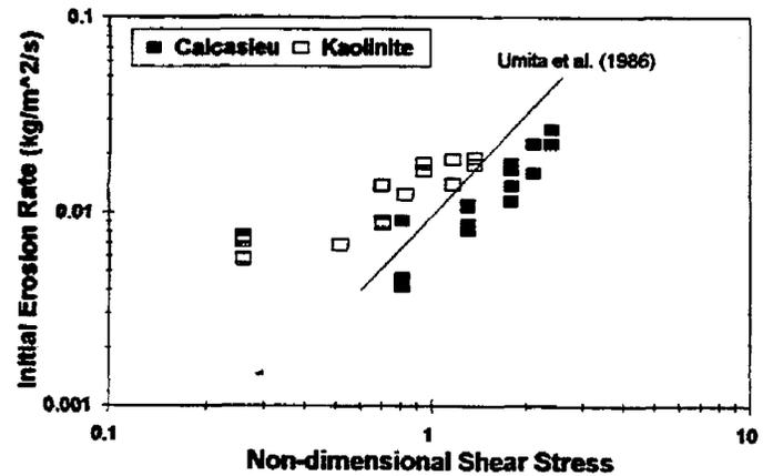
Figure 5. Variation of initial erosion rates with non-dimensional shear stress.
