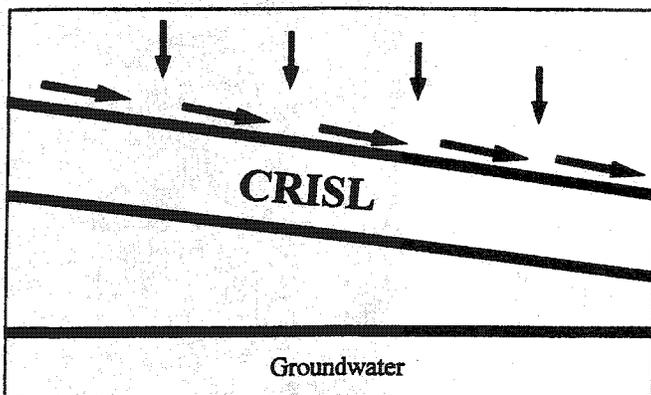
Figure 3. Movement of recharge water and contaminants on continuous CRISL.
