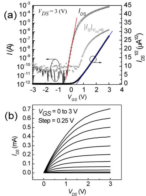
FIG. 2. (Color online) Operation characteristics of sputtered *a*-BST/*a*-IGZO TFT with  $L=5 \mu\text{m}$  and  $W=1000 \mu\text{m}$ . (a) Transfer characteristics (squares)  $V_{GS}$  was swept from -3 to +3 V at  $V_{DS}=3$  V and leakage current (triangles) at  $V_{DS}=0$  V. (b) Output characteristics.  $V_{DS}$  was swept from 0 to +3 V at each  $V_{GS}$  varied from 0 to 3 V at 0.25 V steps.
