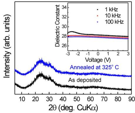
FIG. 1. (Color online) XRD patterns of *a*-BST film on glass substrate as deposited at room temperature and after annealing at 325 °C for 1 h. Inset: Dielectric constant measured on a Au/Ti/*a*-BST/ITO/glass sample as a function of bias voltage and at 1, 10, and 100 kHz.
