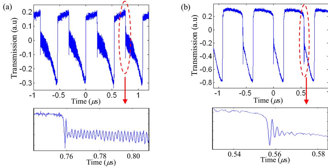
Fig. 2: Experimental results for a microdisk resonator with parameters given in Fig. 1. (a) Top: Observation of simultaneous steady-state MHz thermal and long-sustained GHz oscillations. Bottom: A zoomed view of the GHz oscillations which has a frequency of 0.52-0.54 GHz. The oscillation is sustained for over 110 periods. (b) Top: Observation of simultaneous steady-state MHz thermal and damped GHz oscillations. Bottom: A zoomed view of the damped GHz oscillations in the specified zone.
