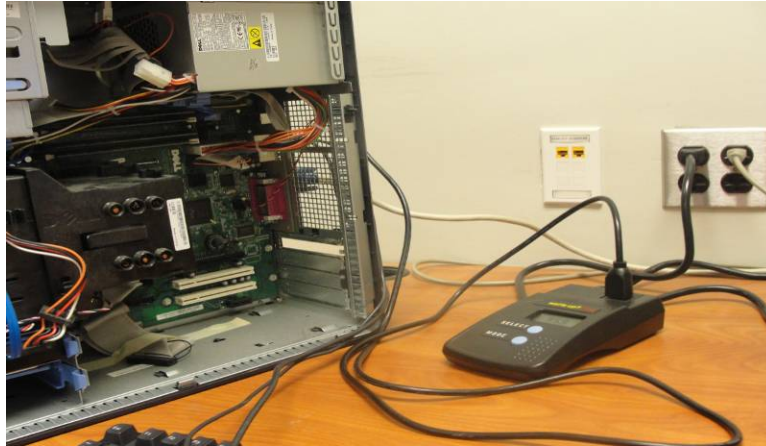
Figure 2-3 Watts up Meter monitoring the AC input power of Desktop Computers
