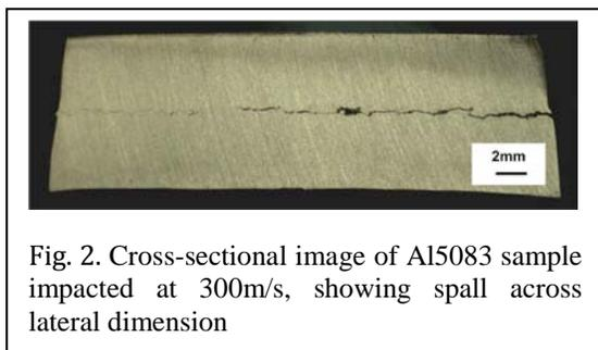
Fig. 2. Cross-sectional image of Al5083 sample impacted at 300m/s, showing spall across lateral dimension
