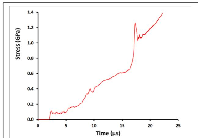
**Fig. 12.** Simulated stress history for a representative Al-5083 sample with SiC hollow spheres subjected to plate impact at 416m/s.
