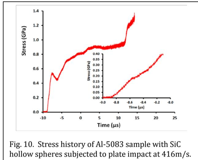
Fig. 10. Stress history of Al-5083 sample with SiC hollow spheres subjected to plate impact at 416m/s.
