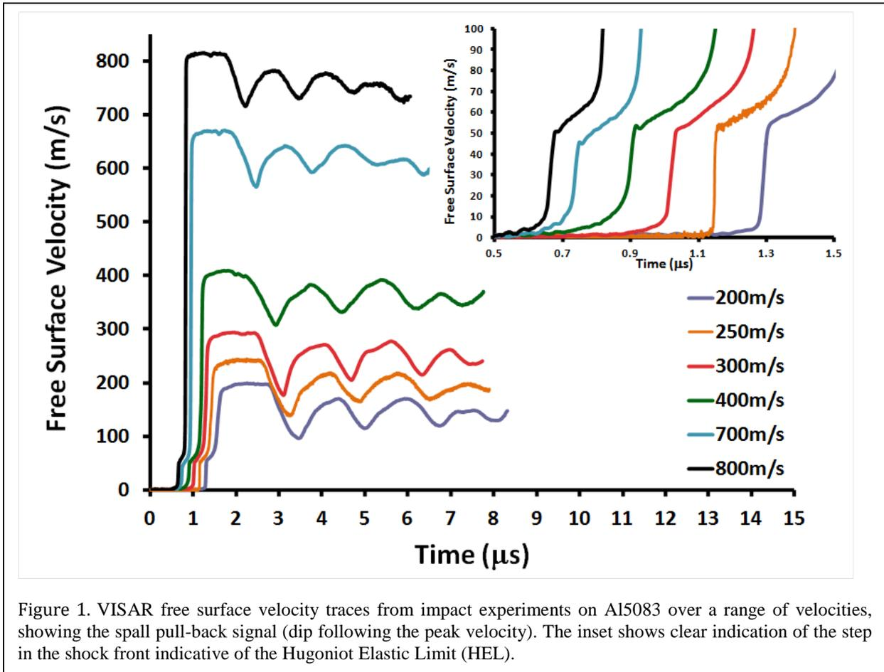
Figure 1. VISAR free surface velocity traces from impact experiments on Al5083 over a range of velocities, showing the spall pull-back signal (dip following the peak velocity). The inset shows clear indication of the step in the shock front indicative of the Hugoniot Elastic Limit (HEL).
