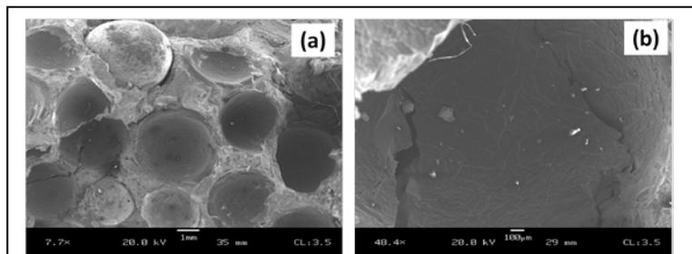
**Figure 9.** SEM images of the fracture surface of the hollow sphere composite sample. The sample fails due to interfacial cracking after penetration by a 0.30 caliber bullet.
