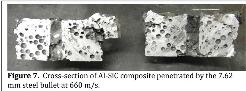
**Figure 7.** Cross-section of Al-SiC composite penetrated by the 7.62 mm steel bullet at 660 m/s.
