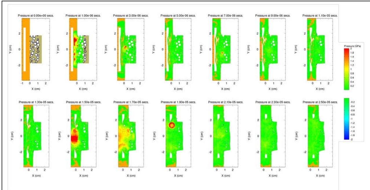
**Figure 11.** Simulated material response of Al-5083 sample with SiC hollow spheres subjected to plate impact at 416m/s. The change in pressure with time throughout the material is also shown.
