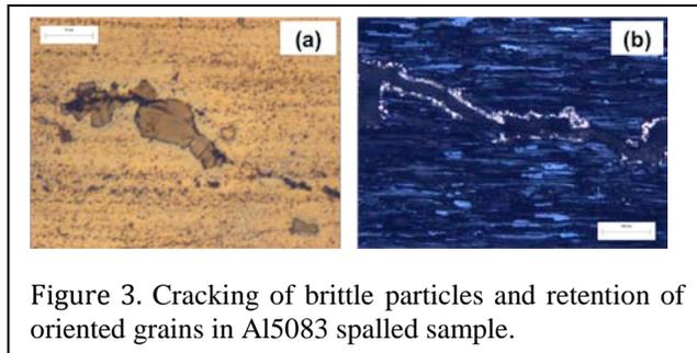
Figure 3. Cracking of brittle particles and retention of oriented grains in Al5083 spalled sample.
