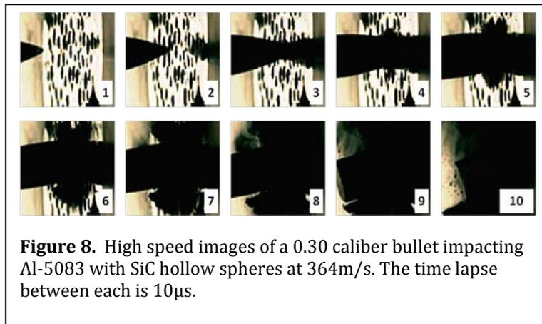
**Figure 8.** High speed images of a 0.30 caliber bullet impacting Al-5083 with SiC hollow spheres at 364m/s. The time lapse between each is 10 $\mu$ s.
