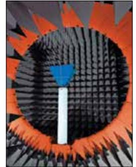
The SG 24 can perform both TRP and TIS measurements according to the CTIA 3.2 test plan.
