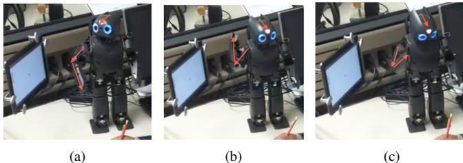
Fig. 3. The fast arm gesture broken down into three parts. (a) Initial Position - Darwin is standing and has eye contact with the tablet-based test. (b) Darwin's right arm is raised, and eye contact is towards the student. (c) Darwin's arm is brought down at a fast speed, and his head follows this downward motion. He then returns to the initial position.
