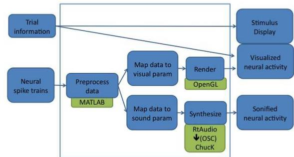
Figure 1: Schematic system diagram.
