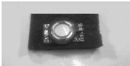
Figure 5: Wearable PCB board with loudspeaker
