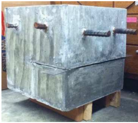
Figure 5.1: Concrete specimen with reinforcement bars and artificial crack.
