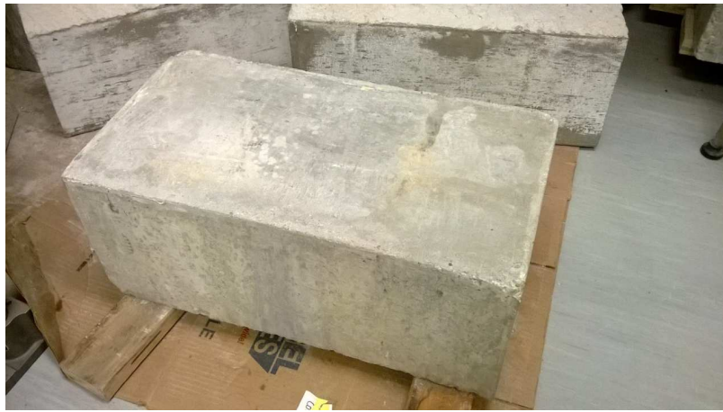
Figure 5.3: Concrete specimen for surface-breaking crack characterization.
