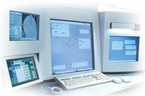
Figure 1. The visual display and computer interface used for air traffic control consoles in Australia.
