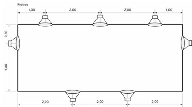
Figure 3. Loudspeaker placement on *DigiWall*
