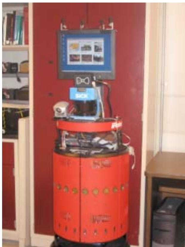
Figure 1. A mobile iRobot B21R configured with microphones, an amplified loudspeaker, and a visual display to function as an information kiosk.
