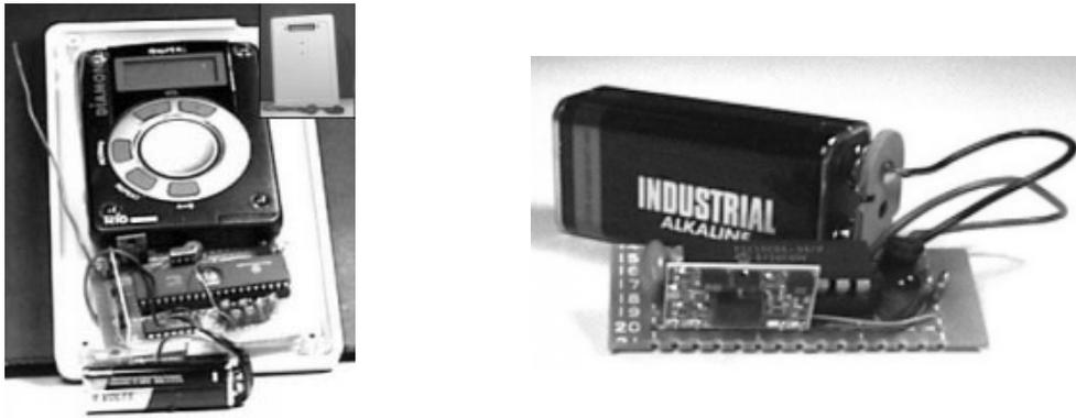
Figure 1: **Left** - The inside of the wearable device showing the Diamond Rio<sup>TM</sup>, the RF receiver, the PIC microcontroller and a 9V battery. The inset is the closed unit. **Right** - The RF transmitter attached to a 9V battery.
