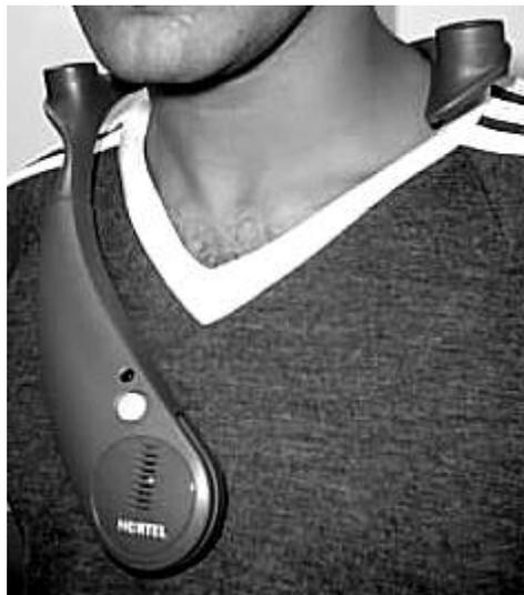
**Figure 2:** The wearable audio device, the *Soundbeam*, with directional speakers and microphone
