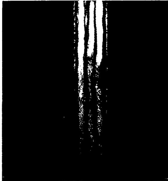
Figure 6. Trajectory of 5.9  $\mu\text{m}$  rayon fibers at 1% consistency and 2.5 cm /s flow velocity.
