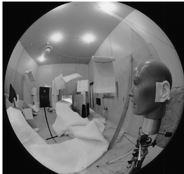
Figure 4. Fish-eye view of the reverberation room in its least reverberant condition, showing the JBL 4206 loudspeaker on the left, and the dummy head on the right.
