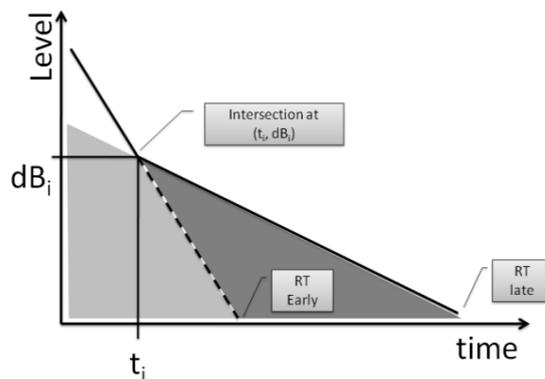
Figure 3. Illustration of a non-exponential decay profile as typical for coupled rooms (see also text).
