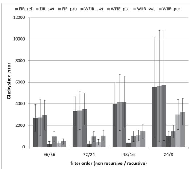
Figure 8: Averaged values of Chebyshev error for all tested filters. Value of standard deviation is marked on every bar.
