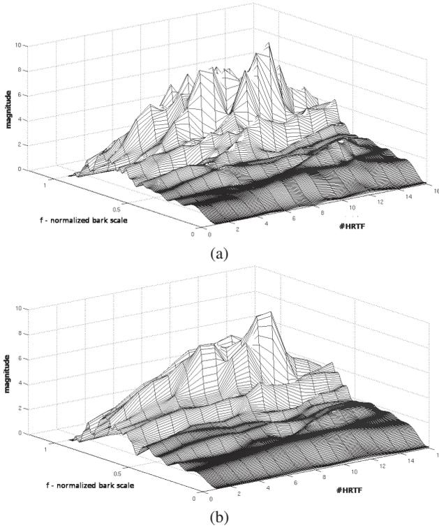
Figure 5: HRTF magnitude spectra for one azimuth angle and sixteen elevation angles - (a) - original data, (b) - reconstructed with four principal components
