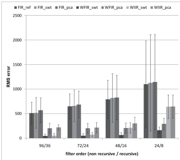
Figure 7: Averaged values of the rms error for all tested filters. Value of standard deviation is marked on every bar.
