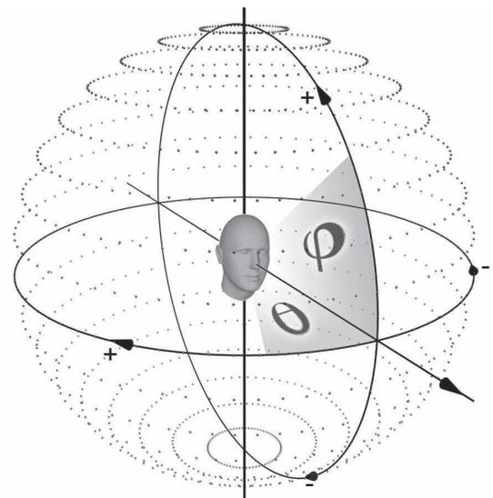
Figure 1: Vertical-polar coordinate system with azimuth ( $\theta$ ) and elevation ( $\varphi$ ) angles highlighted
