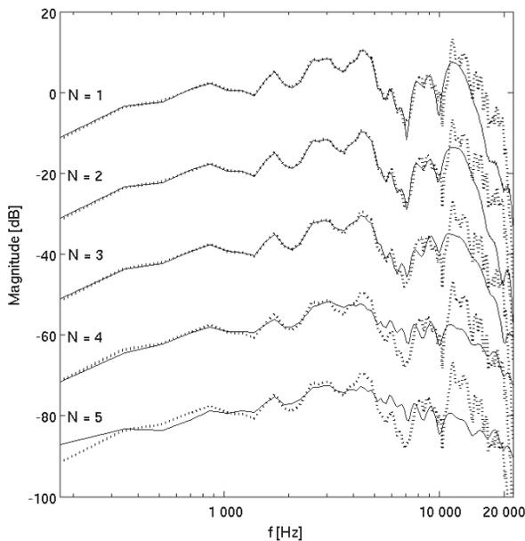
Figure 4: The HRTF magnitude spectra approximated using SWT coefficients for different levels of decomposition. The dotted line is the original magnitude spectrum. For better readability the plots are shifted by 20dB.
