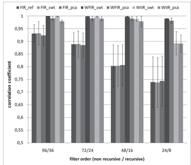
Figure 6: Averaged values of the correlation coefficient for all tested filters. Value of standard deviation is marked on every bar.
