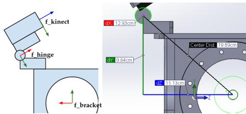
Figure 4: The three frames in play and the transformation from the bracket to the Kinect hinge
