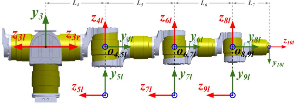
Figure 3: The left arm frames, the torso and the base of the right arm
