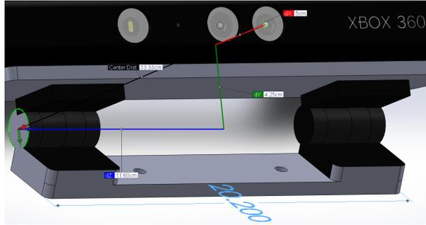
Figure 5: The transformation between the Kinect hinge and the 3D sensor lens
