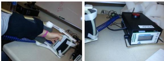
Figure 1. Hand Mentor arm brace (left) and control box (right).
