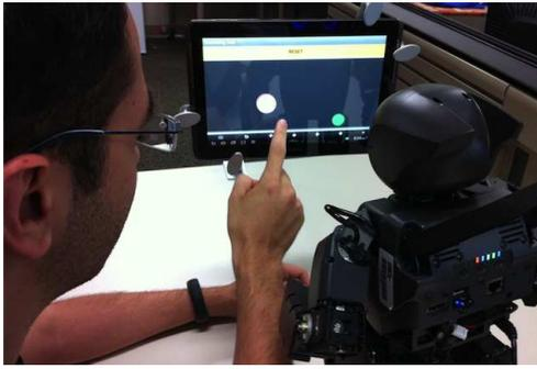
**Figure 4: A touchscreen tablet computer will function as a shared workspace for human-robot collaborative task solving.**
