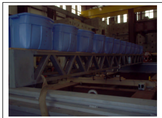
Figure 2. Simulated Uniform loading
