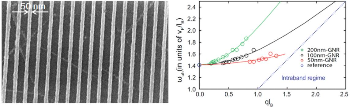
**Figure 1:** (Left panel) Scanning electron microscopy image of a 50nm-wide GNR array sample. (Right panel) Dispersion relation of the UHM,  $\omega_{uh}(q l_B)$ , in units of  $v_F/l_B$ , where  $\omega_{uh}$  is the UHM frequency,  $q$  is the in-plane wave vector,  $v_F$  is the Fermi velocity, and  $l_B$  is the magnetic length.
