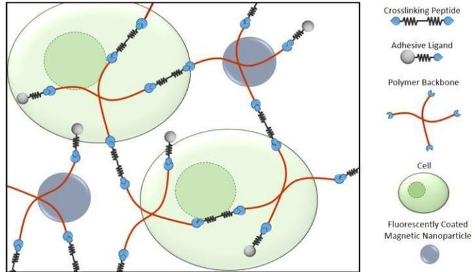
**Fig 3:** Hydrogel components and cross linking effect under the influence of fluorescent-magnetic nanoparticles.
