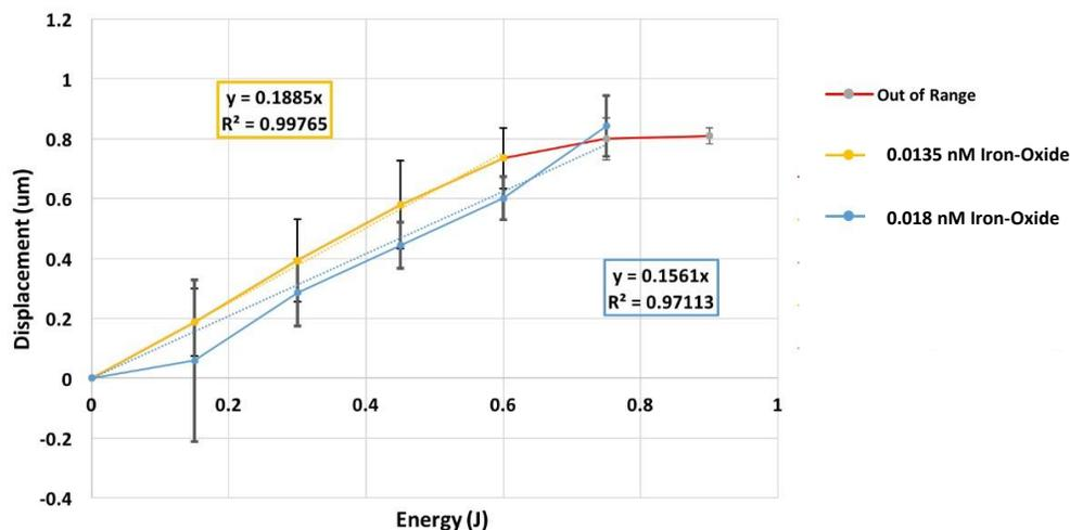
**Graph 2:** Displacement vs. number of magnets. Displacement increases linearly with number of magnets for both 0.0135 nM and 0.018 nM iron-oxide particle concentration.
