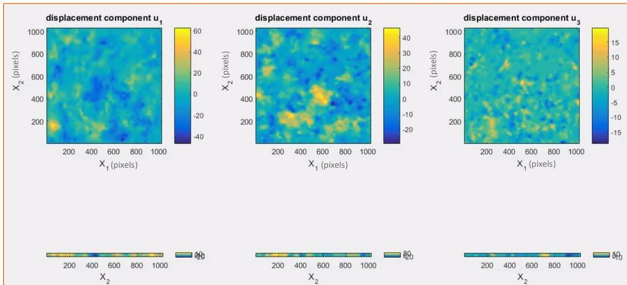
**Fig 2:** Fast Iterative Digital Volume Correlation (FIDVC) program output window that displays the deformation from an external permanent magnet as pixel movement according to an axis. Movement in the  $u_1$ ,  $u_2$ , and  $u_3$  direction corresponding to the x, y, and z axis of the 3D stack images. The  $X_1$  and  $X_2$  axis are measured in units of pixels and correspond to the 2D side of the voxel imaged. These pixels contribute to a displacement of  $12.068 \mu\text{m}/\text{pixel}$ .
