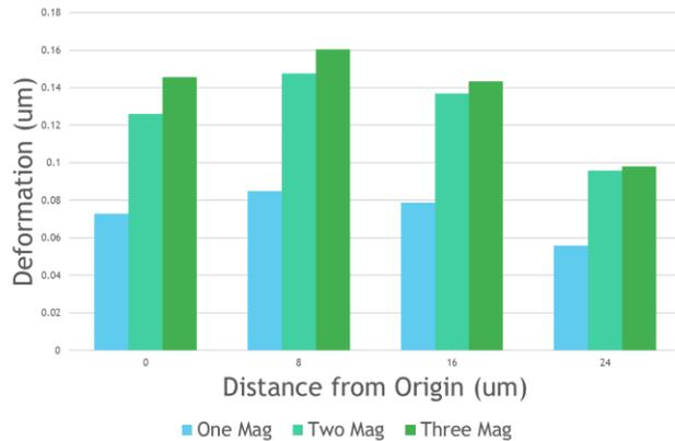
**Graph 3:** Deformation vs. magnet deformation from origin. Displacement increases with an increase with number of magnets.
