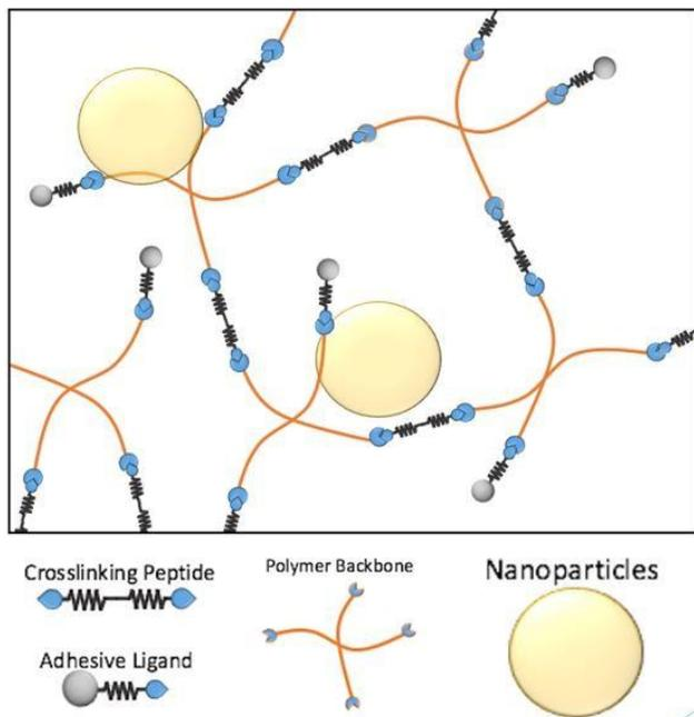
**Fig 1:** Hydrogel components and cross linking effect.
