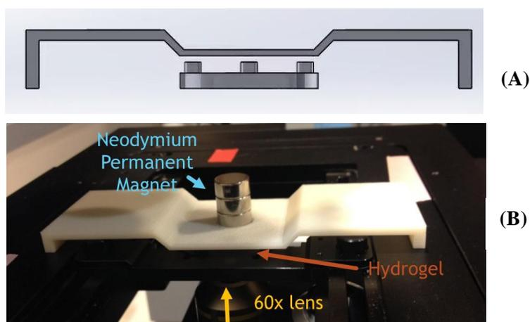
**Fig 4:** Non-magnetic Stage for confocal microscope (A) Solid Works design (B) 3D Printed design placed on confocal microscope.
