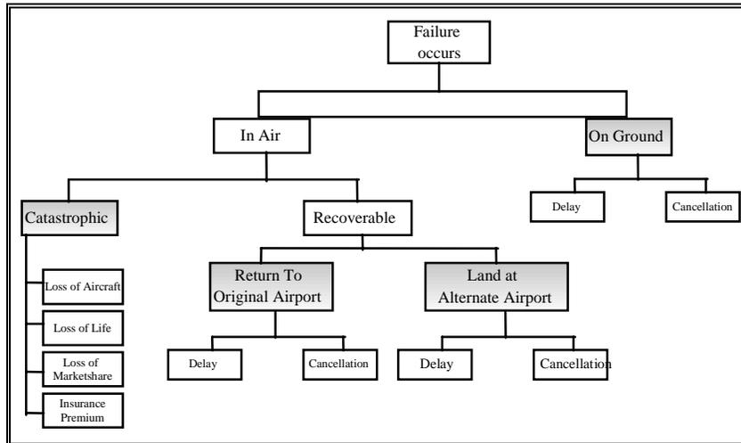
**Figure 2: Four Main Types of Failure Modeled in The Revenue Loss Module Within ALCCA**
