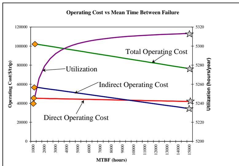
**Figure 9: Operating Cost Versus Mean Time Between Failure**
