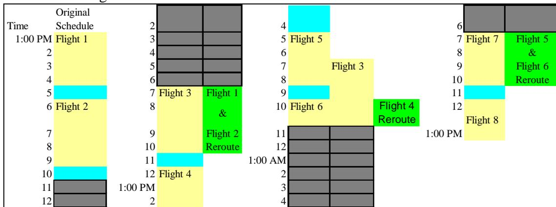
**Figure 5: Example of Day 2, Overnight Flight Rescheduling: Block Time = 4 hrs, Ground Time = 1 hr, Daily Utilization = 16 hrs, MTTR = 28 hrs**
