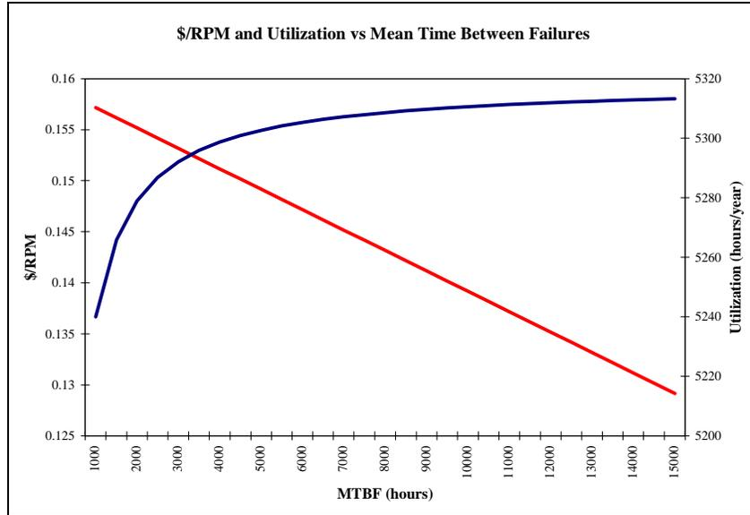
**Figure 8: \$/RPM and Utilization versus Mean Time Between Failures**
